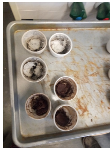
FIGURE 32. Samples after burning dry matter, in 550 °C, for 2 hours (Qiuwang Fan 2018)
