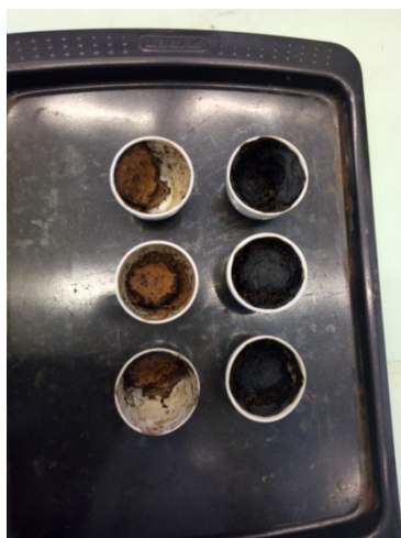
FIGURE 31. Samples after drying fresh matter, in 105 °C, for 20 hours (Qiuwang Fan 2018)
