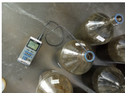
FIGURE 42. Measuring pH of reactor (Qiuwang Fan 2018)
