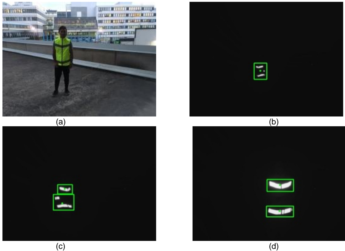
Figure 24. a. Color image taken from external camera. b,c,d. Real-time verification results in outdoor conditions during evening time
