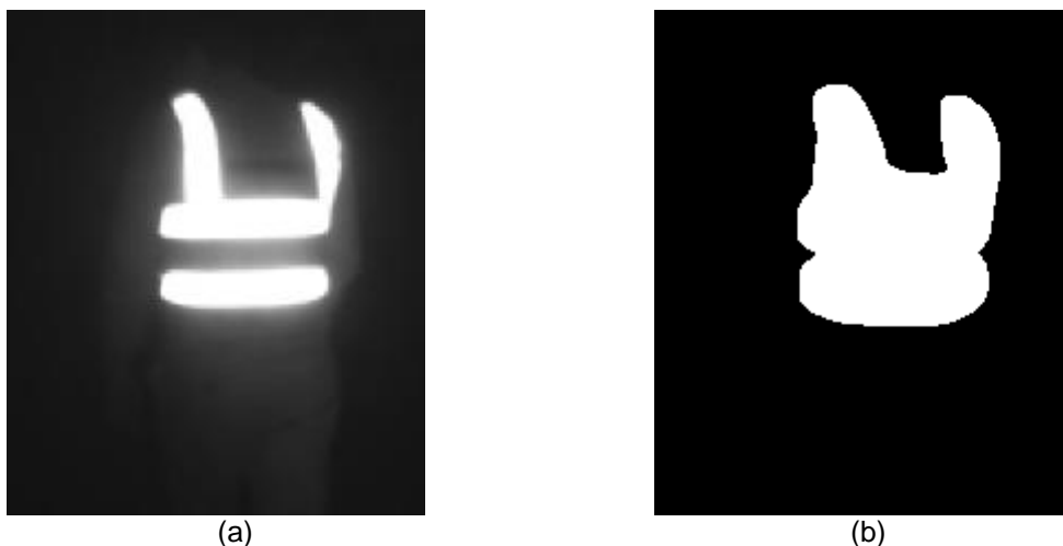
Figure 8. a. Raw image taken with flash / b. Resulting image after thresholding and dilation
