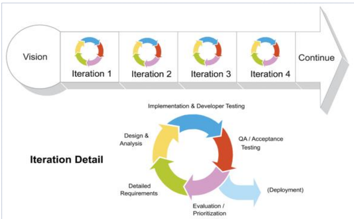
Figure 9. The fixed intervals of Scrum Sprints by blending all the phases together for each interval. (James, 2015).
