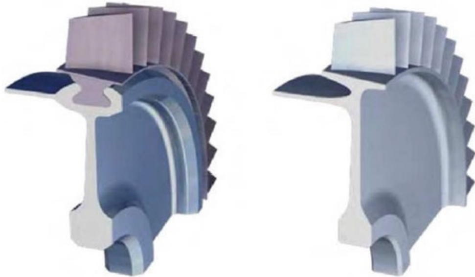
Figure 23. Conventional bladed-disc and blisk. Left: mechanical attachment of blades, right: blades are welded (10, p. 300)
