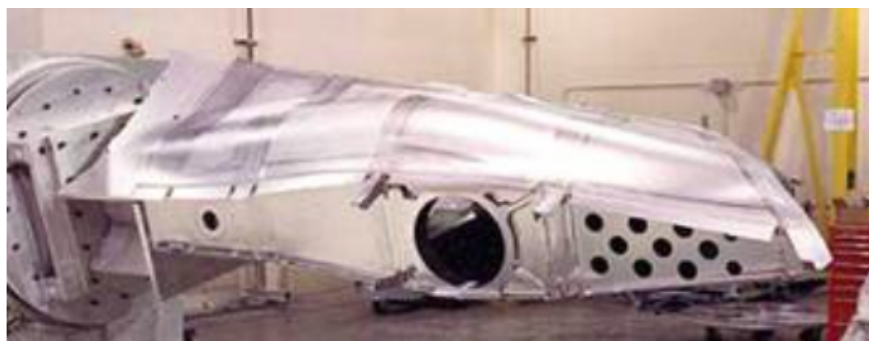
Figure 67. Welded aft boom (3, p. 50; 65, p. 54)
