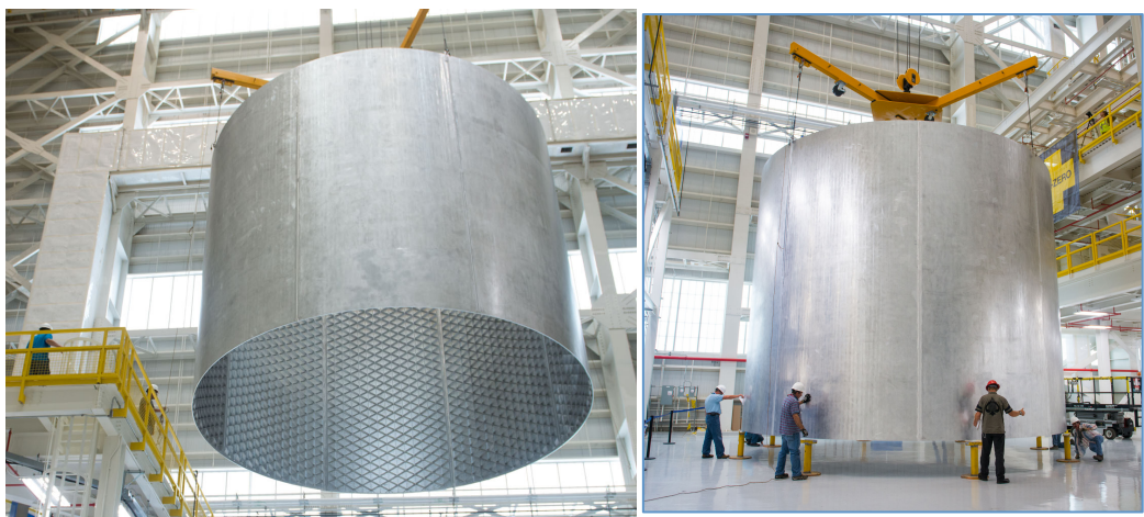
Figure 18. Fully welded SLS barrel section for the liquid hydrogen tank (13)
