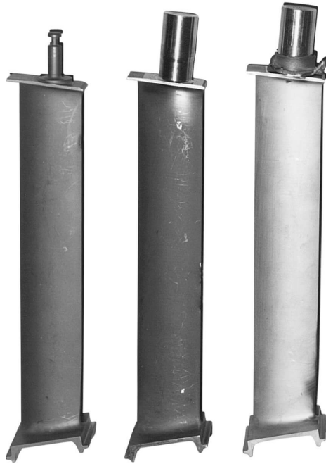
Figure 34. Left: stator vane root weld – as machined, center: stator vane root weld – with flash removed, right: stator vane root weld – as welded (titanium) (37)
