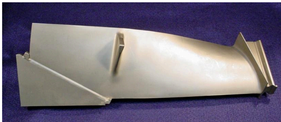
Figure 61. Ti6Al4V fan blade repair with the welded "patch" (62)
