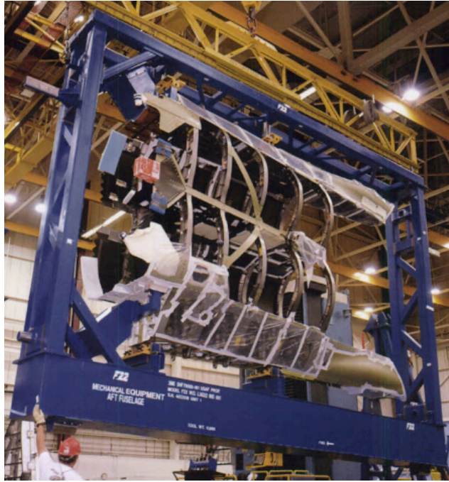
Figure 66. The aft fuselage that support the horizontal tails and some of the vertical tail loads of F-22 (65, p. 51; 67)
