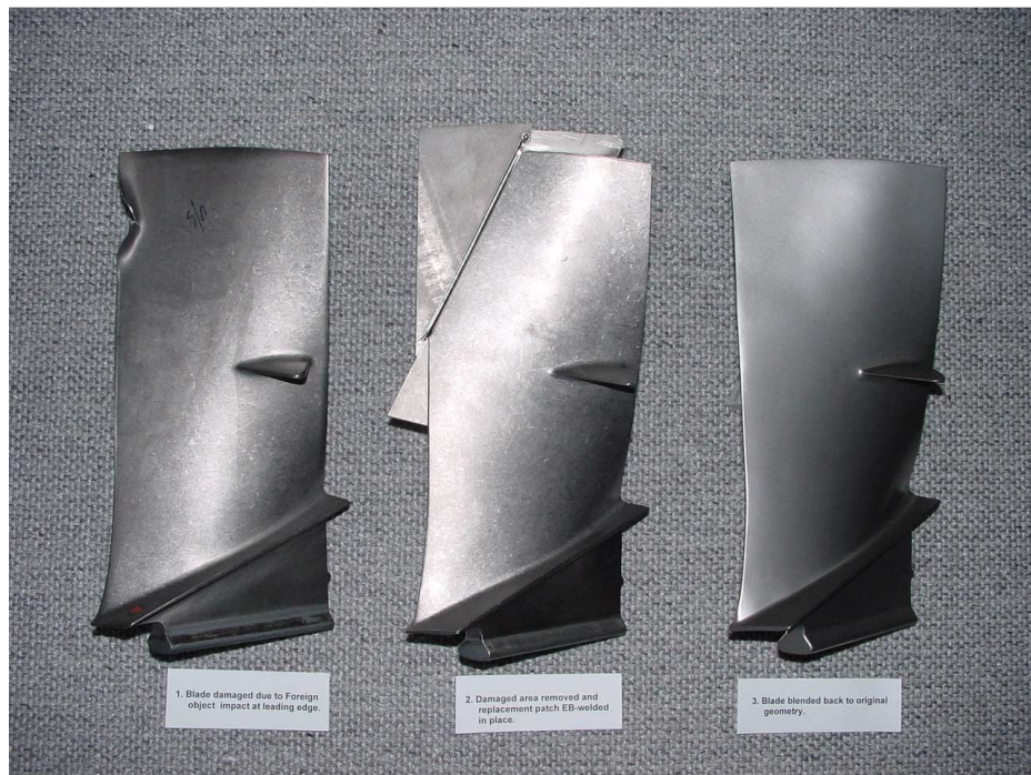
Figure 60. FOD EBW Repair Process of Fan Blades (63)
