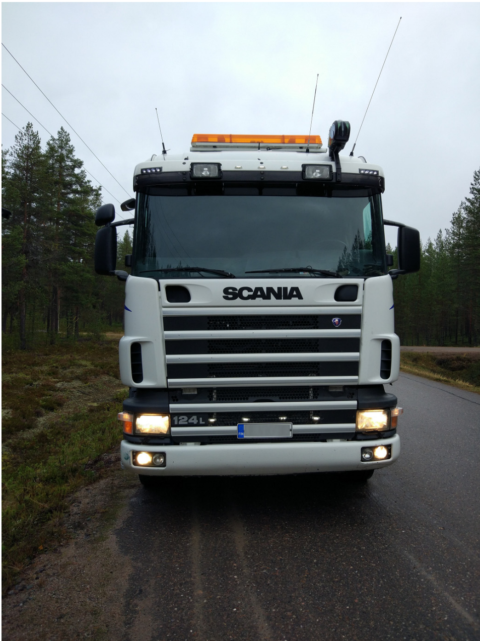
Figure 4 The LGV prime mover used for the tests with the RoadFly mounted to the front.
