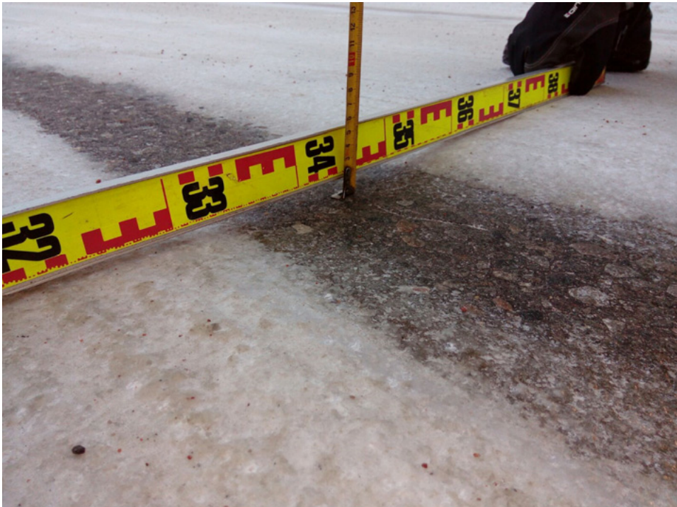
Figure 2 Measuring evenness of hard compressed snow layer (Romakkaniemi, 2018)
