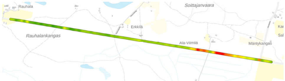
Figure 6 A single test run drawn on the map with the rut colour coding (background map NSL Topographic Database 04/2018)
