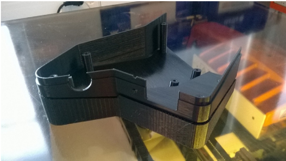
Figure 12 The 3D printed part of the prototype made of PLA material.
