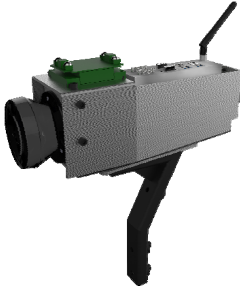
Figure 8 Inner aluminium sheet metal case with separate mounting arm, used in the third and the fourth concepts.
