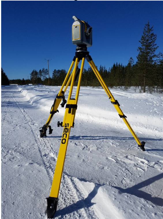
Figure 3 Trimble SX10 scanning total station on position during measurements on 15.3.2018
