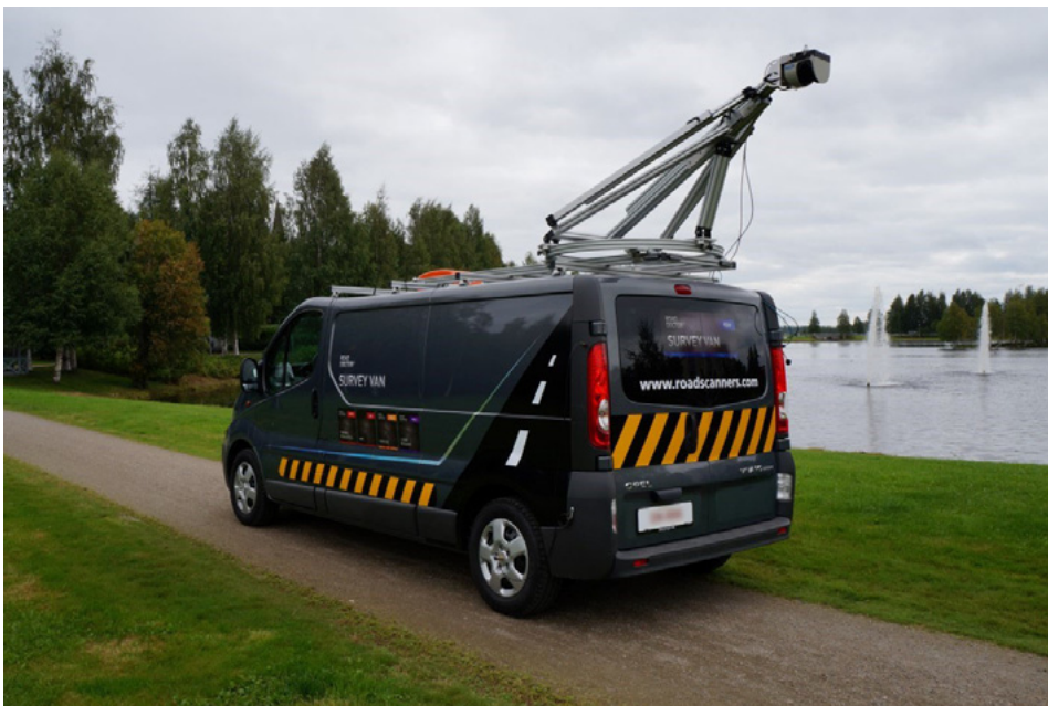
Figure 2 RDSV with the laser scanning unit (Saarenpää 2018)
