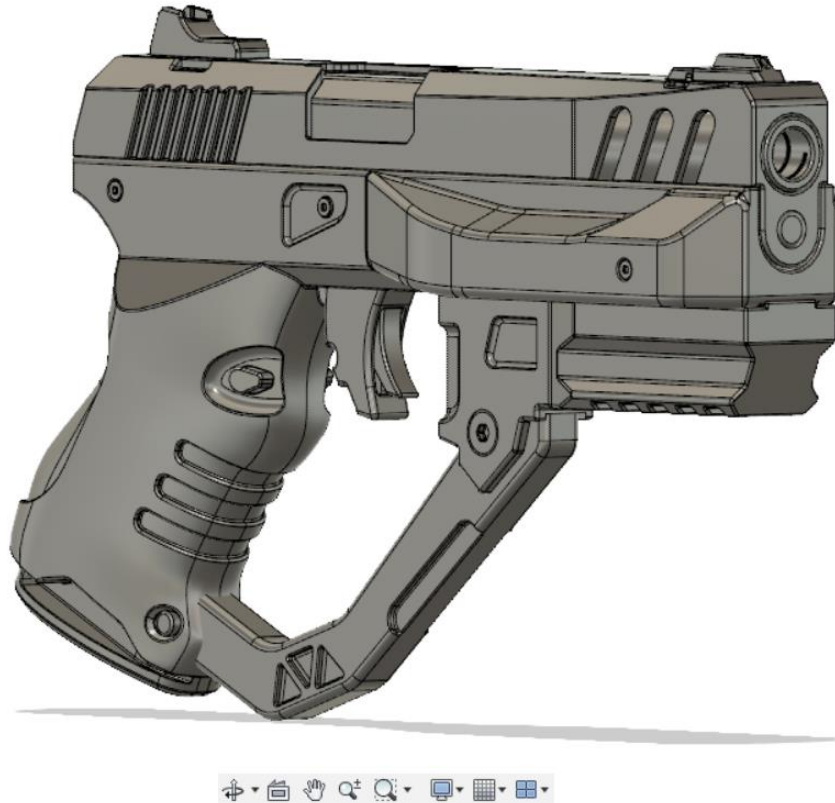
Figure 31. Model with fillets (Kochetov 2018)
