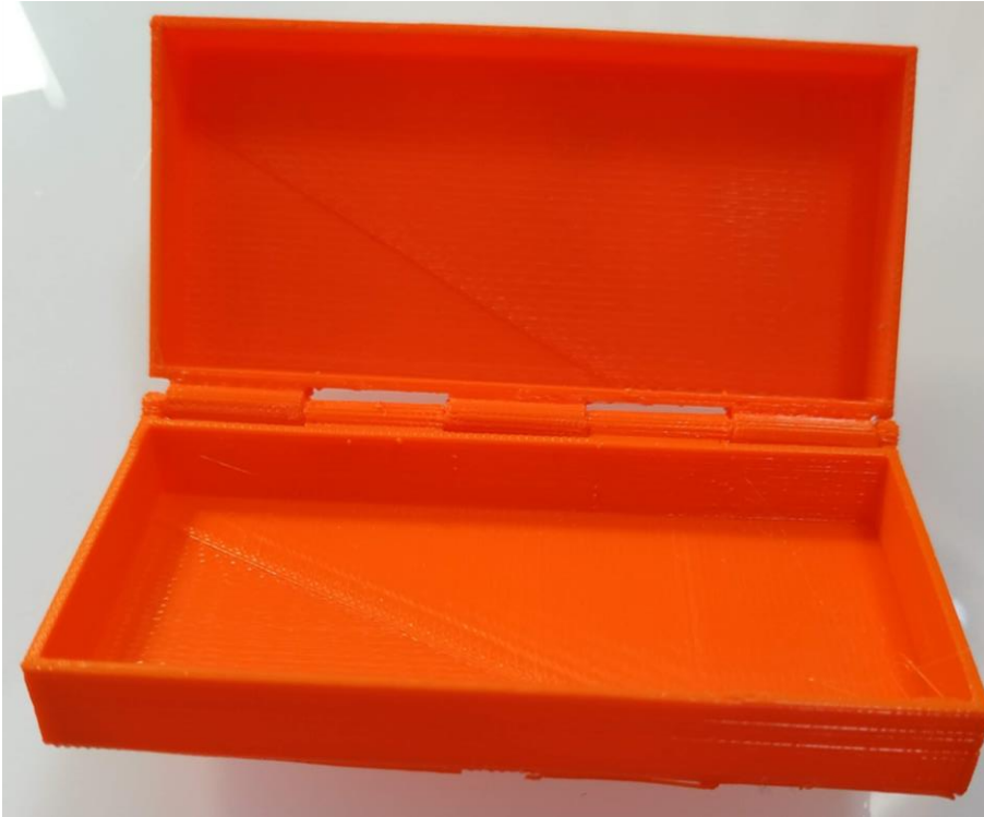
Figure 34. Hinge box modelled in Onshape (raft removed)
