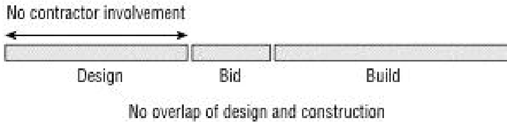
Figure 3.1 Design-Bid-Build Linear approach
