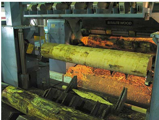
Figure 2.3 Peeling, clipping and stacking line
