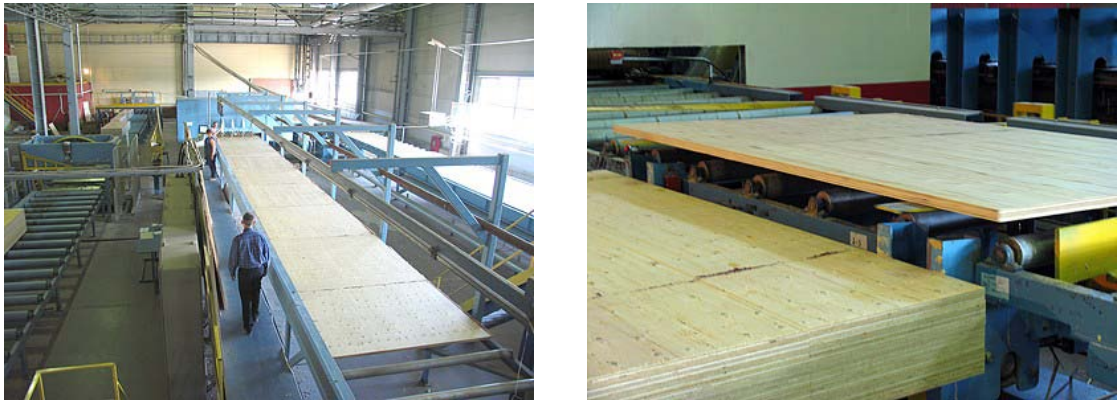
Figure 2.9 Final sizing and grading line
