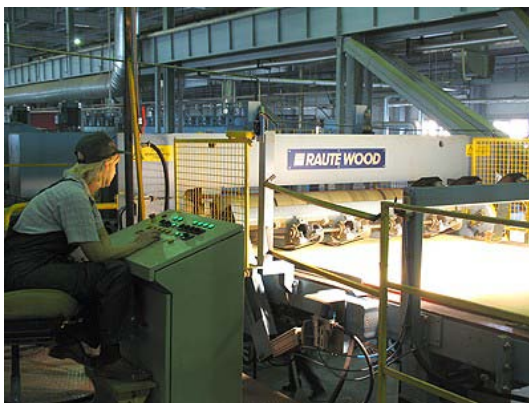
Figure 2.5 Patching and splicing line
