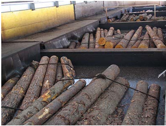
Figure 2.2 The process of hydrothermal treatment and peeling
