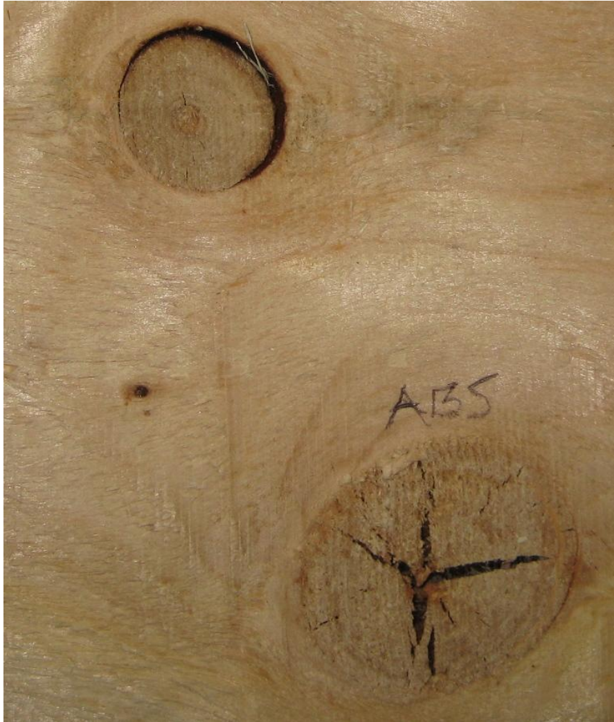
FIGURE 17. Sapwood knots in absolute degree of dryness
