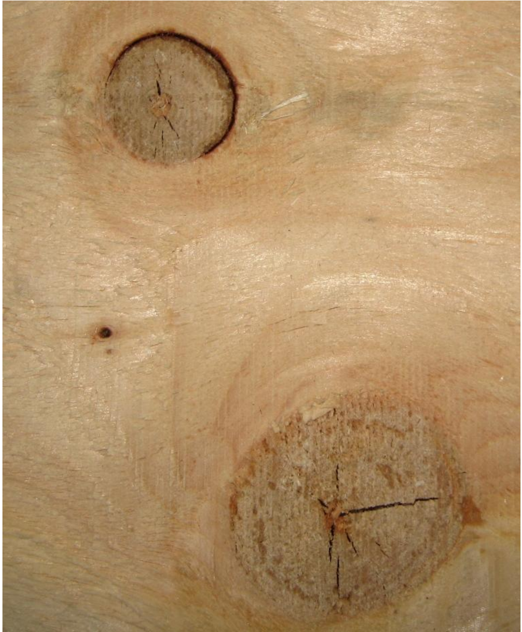
FIGURE 13. Sapwood knots after two and a half hours in the oven
