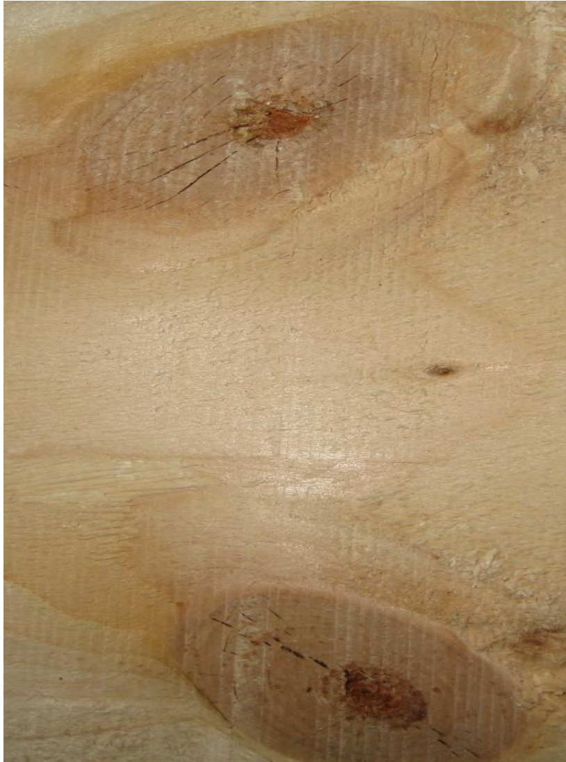
FIGURE 20. Heartwood knots after two and a half hours in the oven
