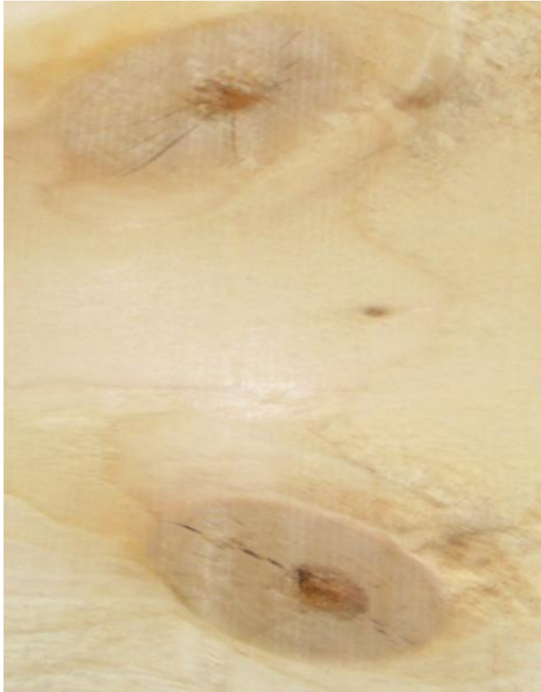
FIGURE 21. Heartwood knots after three and a half hours in the oven
