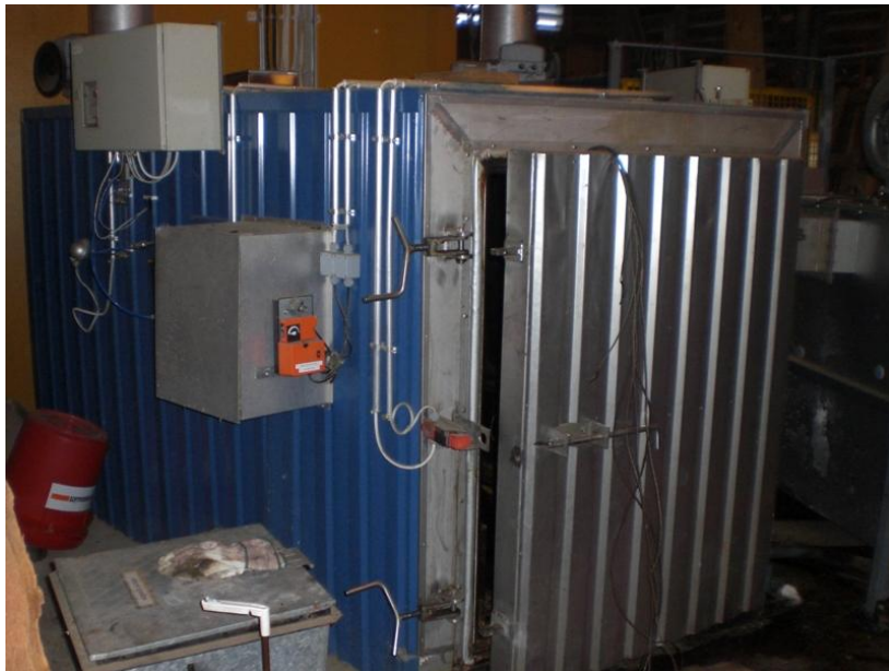
FIGURE 9. Heat treatment kiln by Tekma Wood. (Batch kiln)
