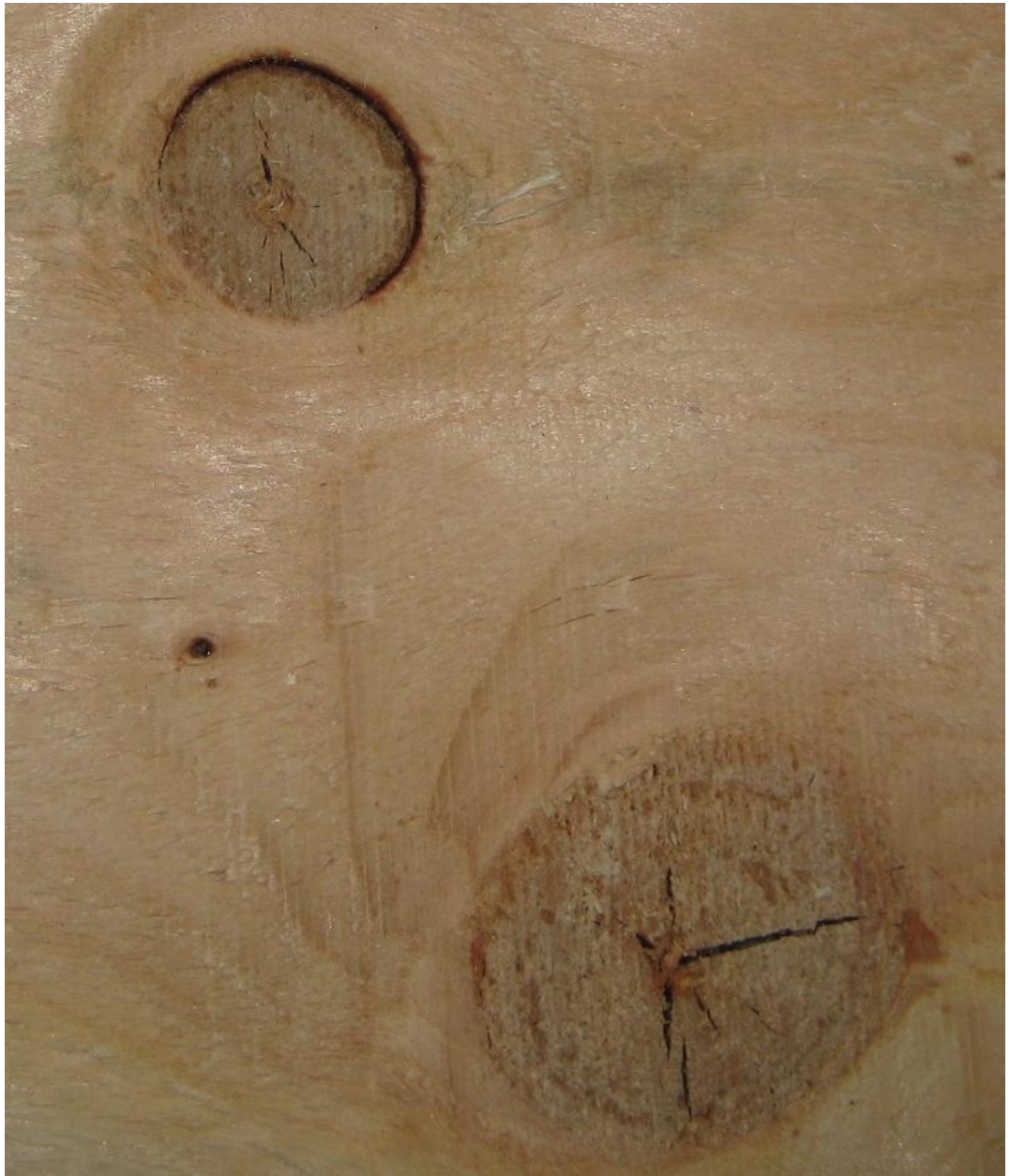
FIGURE 14. Sapwood knots after three and a half hours in the oven
