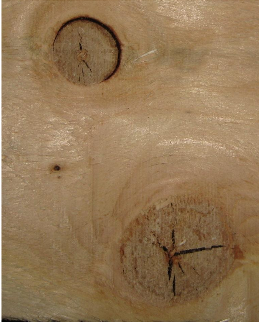
FIGURE 15. Sapwood knots after six hours in the oven
