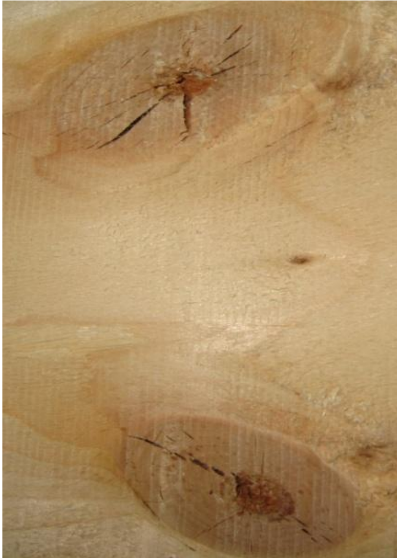
FIGURE 22. Heartwood knots after six hours in the oven
