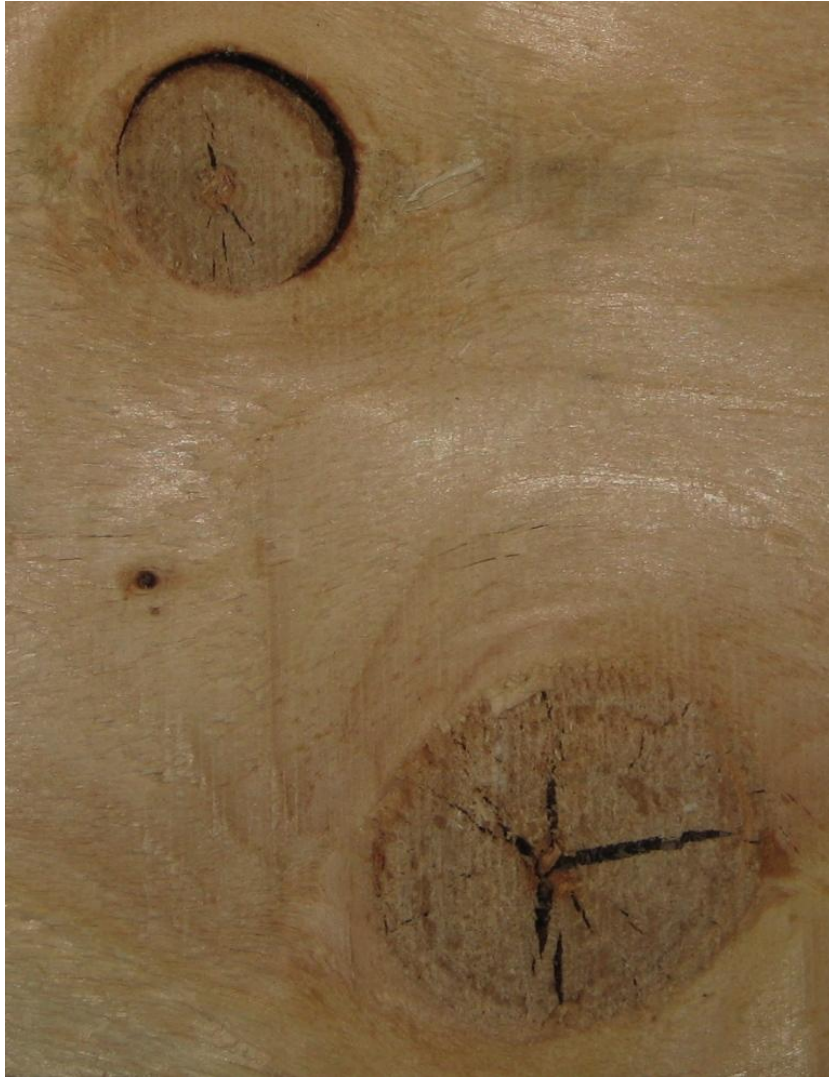
FIGURE 16. Sapwood knots after seven hours in the oven
