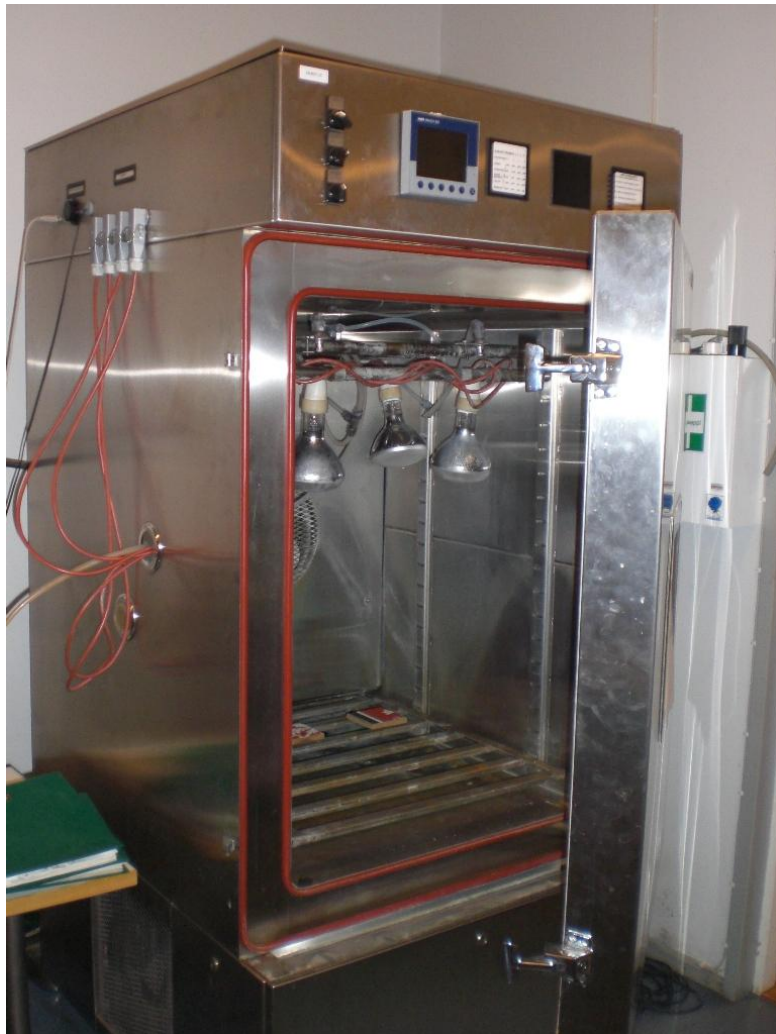
FIGURE 26 . Seasoning chamber where it is possible to simulate real weather conditions.
