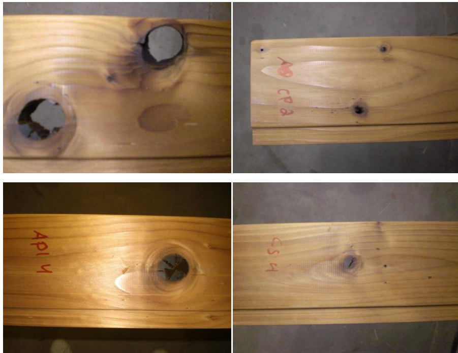
FIGURE 29. Thermally modified Sitka spruce cladding with tongue and groove
