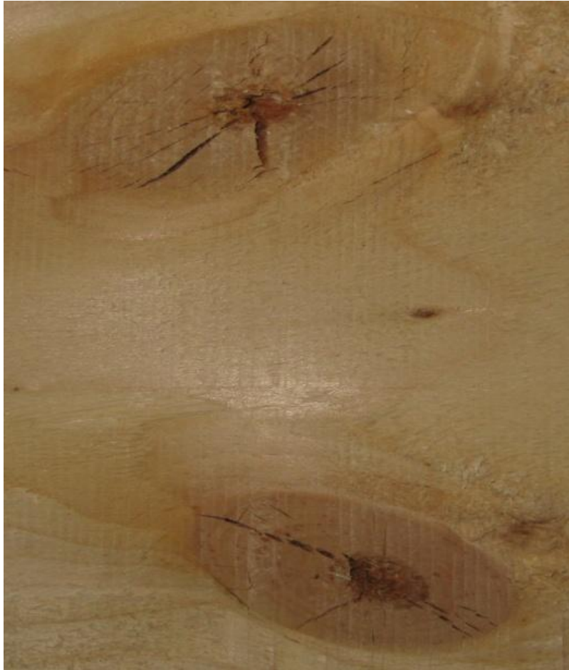
FIGURE 23. Heartwood knots after seven hours in the oven
