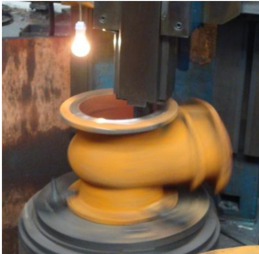
Figure 21. Turning of contact surfaces of the flanges
