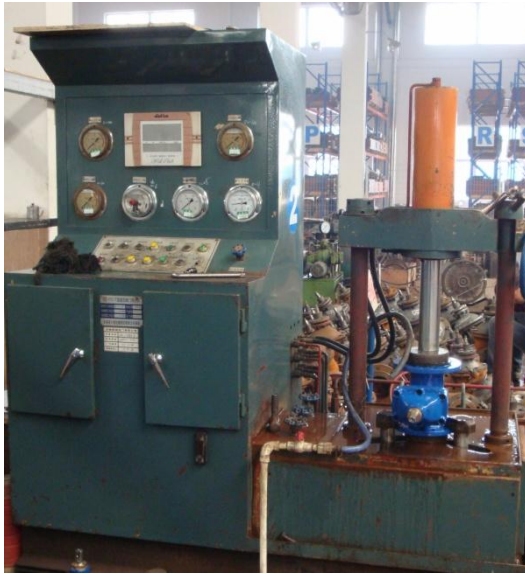
Figure 29. Equipment of pressure test
