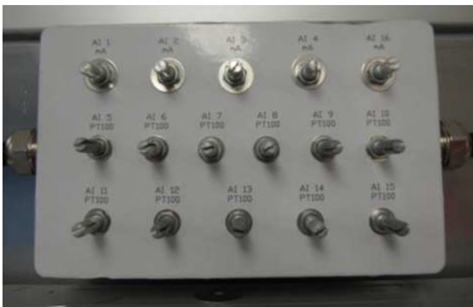
Figure 10. Box with potentiometers for pt100 and mA sensor simulations.
