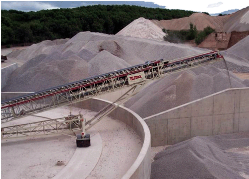
PICTURE 8. Telestack conveyor (Powerscreen Ireland http://www.powerscreenireland.ie/stock/stockpilers.htm )
