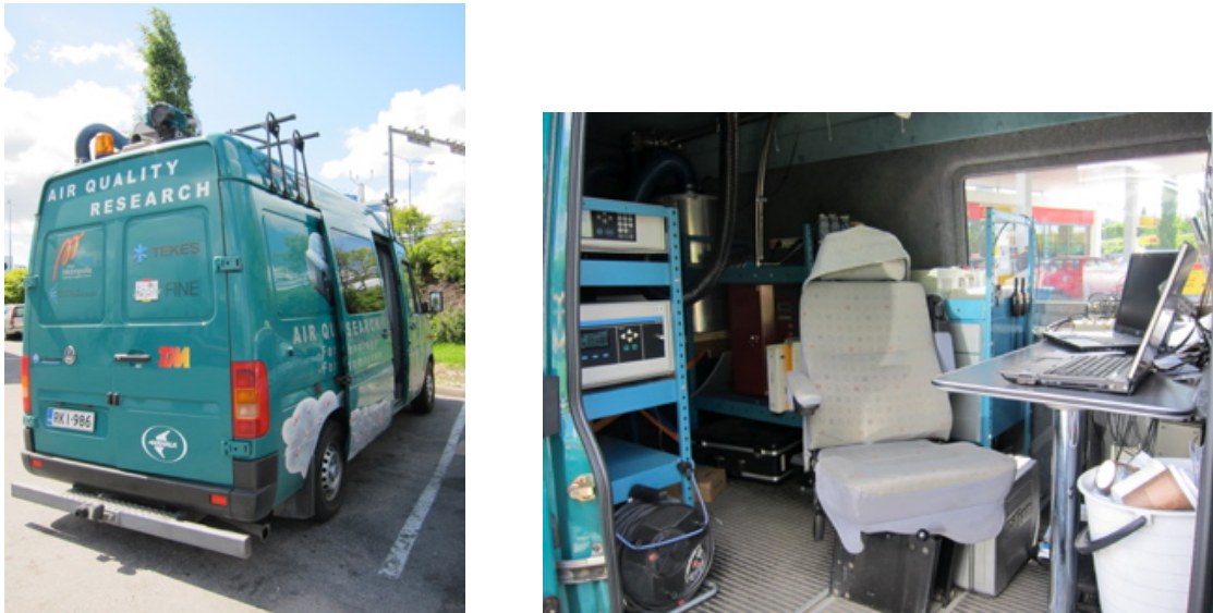
Figure 10. The Sniffer vehicle used in KAPU project to collect PM_{10} emission data from street surface. (Pictures: Roosa Ritola)
