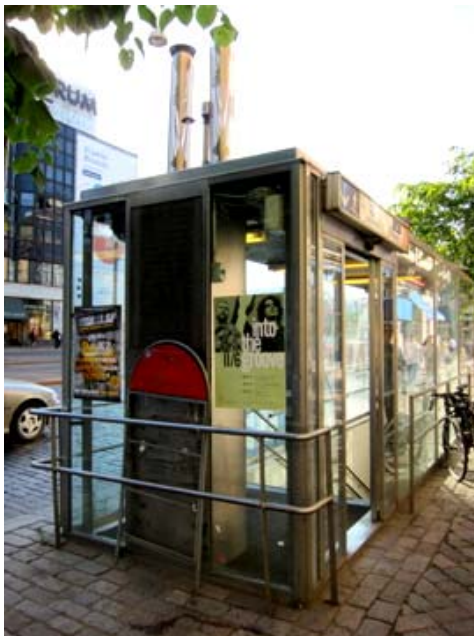
Figure 9. The air quality measuring point in Mannerheimintie, Helsinki city centre (left), is placed on the wall of a glass booth. Measuring station in Pirkankatu, Tampere (right) is placed inside a brick building situated in a small park area between two busy streets. (Pictures: Roosa Ritola)
