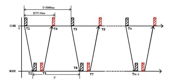
Figure 11. Frames travelling in time domain.
