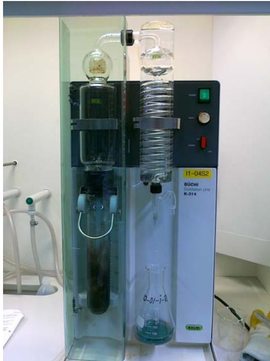
FIGURE 9. Distillation unit K-314 manufactured by Büchi
