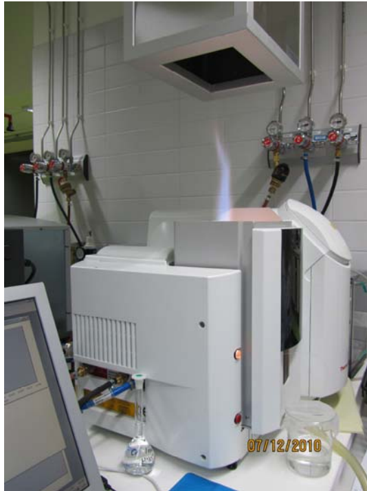
FIGURE 11. SOLAAR M Series AA Spectrometer manufactured by Thermo Scientific
