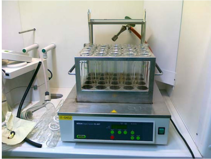
FIGURE 8. Digest system K-437 manufactured by Büchi
