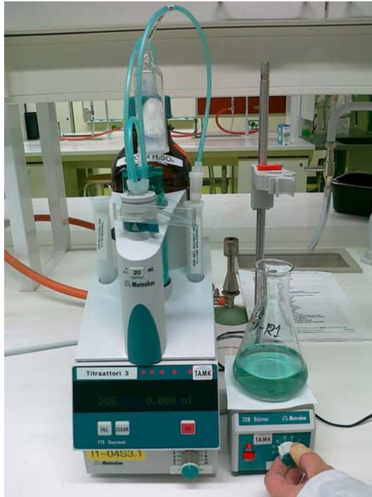
FIGURE 10. Metrohm 775 Dosimat Automatic Burette for Titrator manufactured by Metrohm AG
