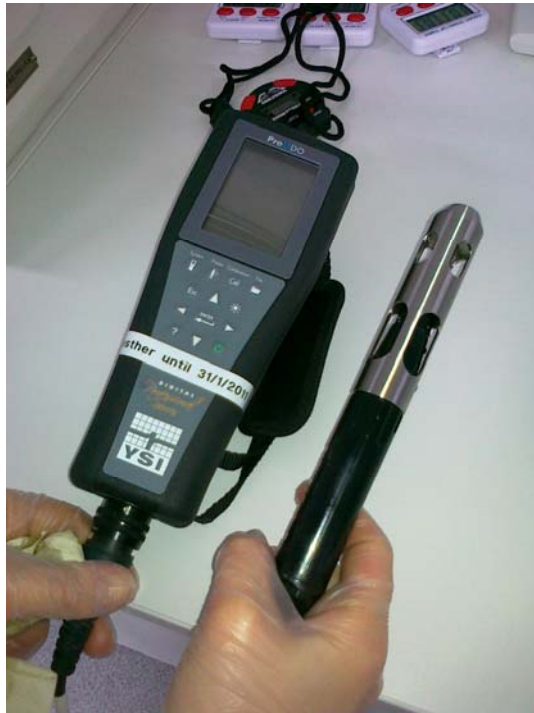
FIGURE 7. YSI Pro ODO™ Handheld Optical DO Meter manufactured by YSI Incorporated
