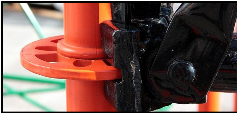
Figure 24 Ring-Lock by RINSTROY, secured on tube by plastic deformation
