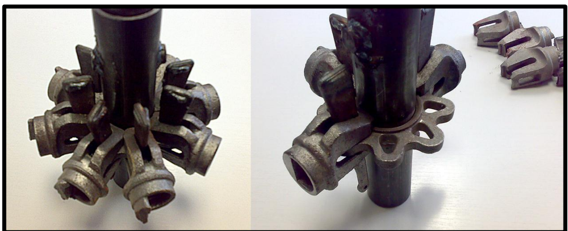
Figure 38 Connection of elements to the «Star» joint
