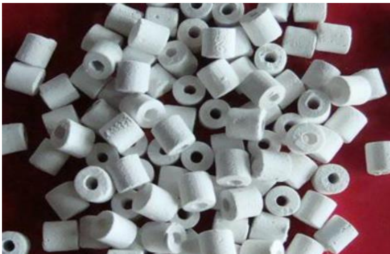
FIGURE 13. Catalyst carrier made of titanium dioxide. (adapted from Lei & Jiang 2001.)
