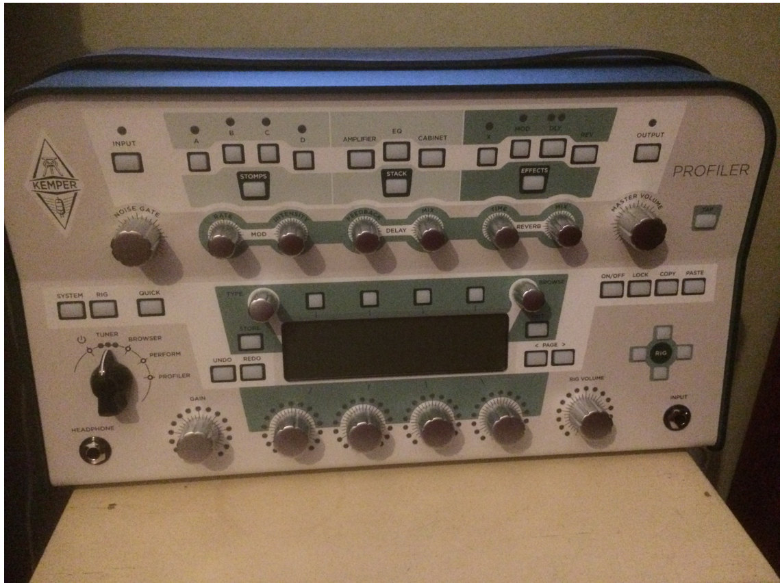
PICTURE 10. A modular guitar amp allow to clone any guitar amp (Hiilesmaa 2020)
