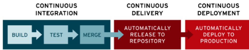
Figure 7. CI/CD pipeline process
