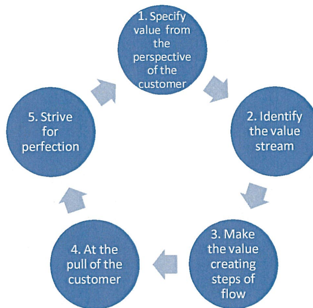
Figure 2. The five key principles of Lean production. (Hines, Peter. Found, Pauline. Griffiths, Gary. Harrison, Richard. 2008, 4).
