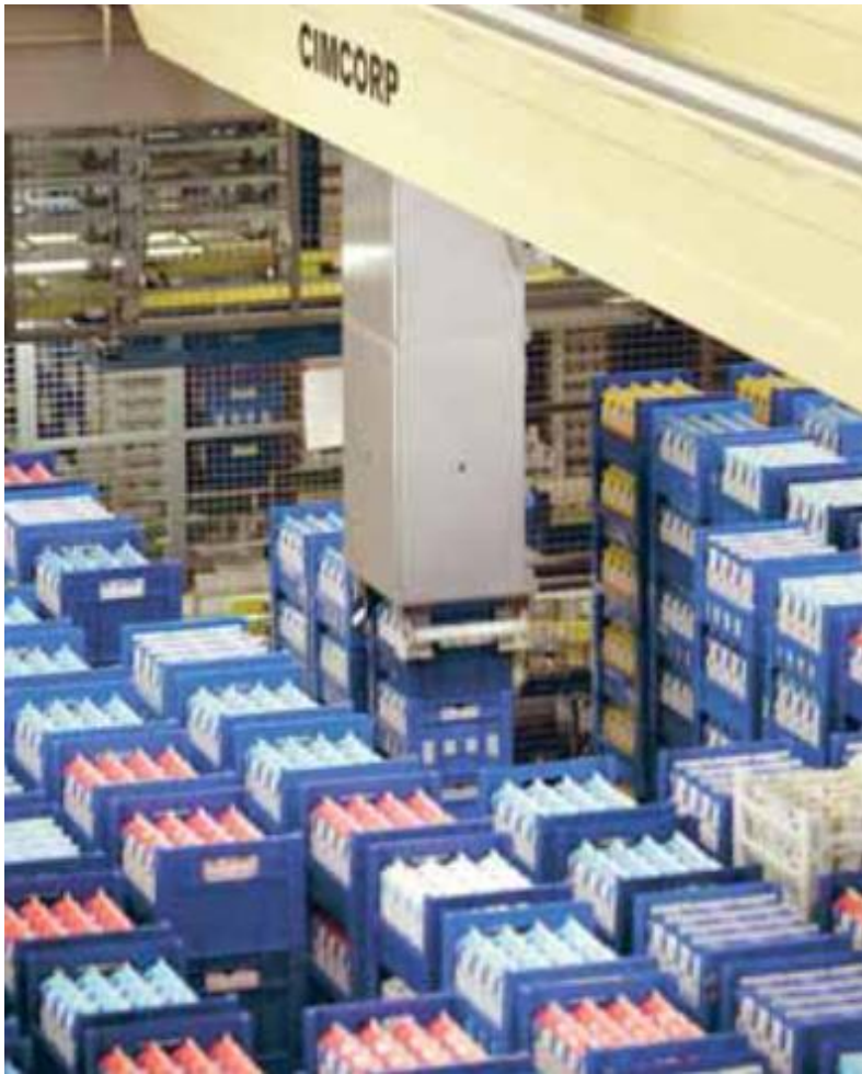
KUVIO 8. MultiPick-robotti (Automated order picking system for dairy products n.d.)
