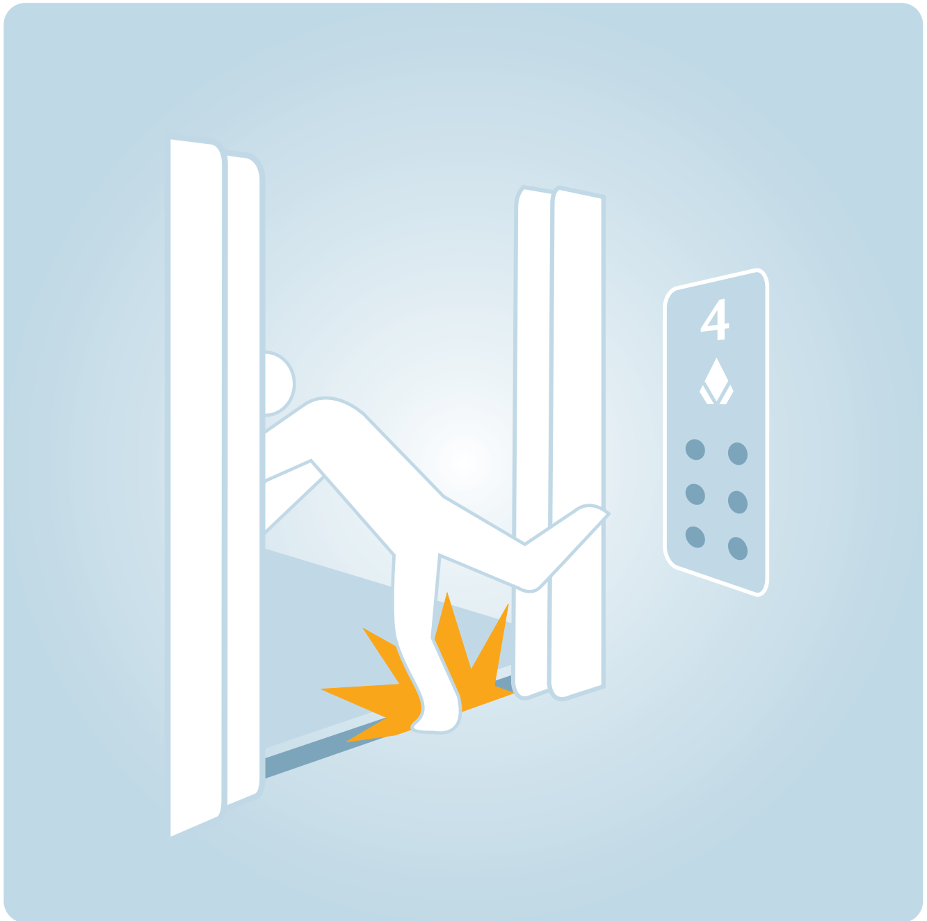
EN 81-80 Hazardous Situation 9: Inadequate vertical surface be- low landing door sills.
