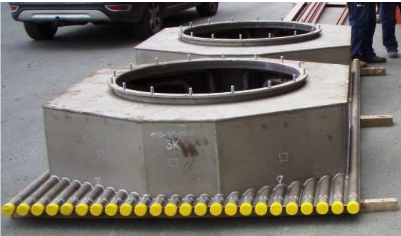
Figure 22. Burner Opening, from outside
