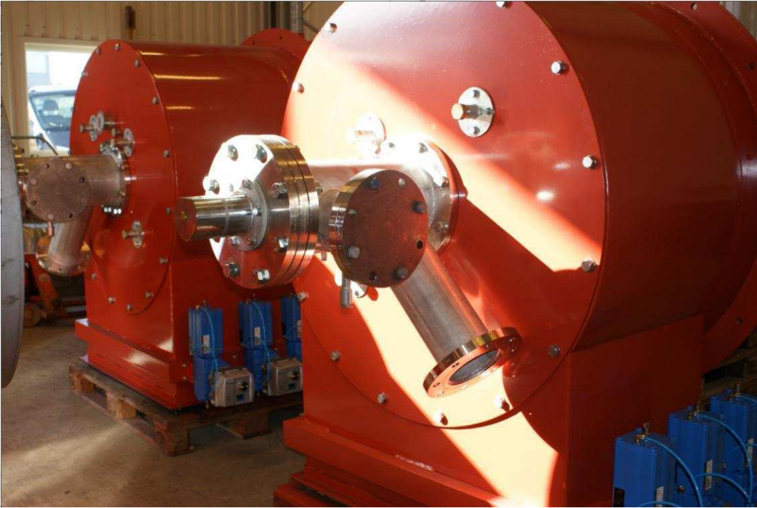
Figure 15. Burners, before installation
