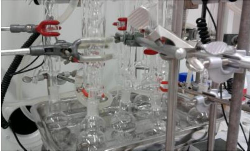
GRAPH 7. The system designed for performing the enzymatic hydrolysis
