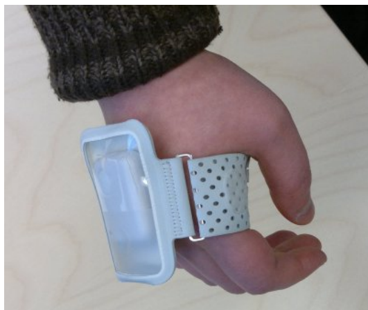
FIGURE 3. Picture of the accelerometer-gyroscope in its container attached to the hand
