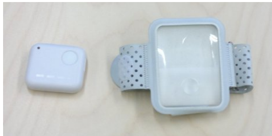
FIGURE 2. Picture of the accelerometer-gyroscope and its container
