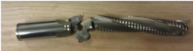
Figure 8. A broken machining tool (ballpoint tool, 16 mm diameter)
