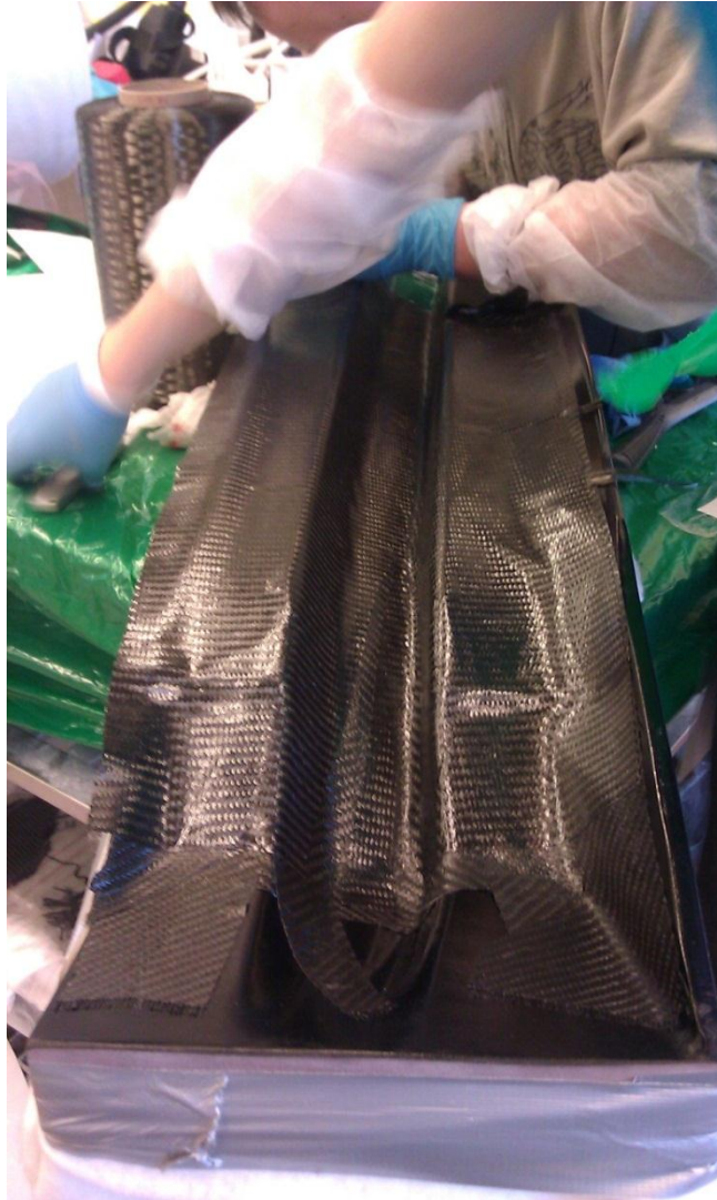
Figure 24. The laying of pre-preg carbon fibre fabric on a mould
