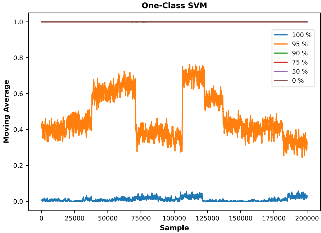
Figure 24. Parameter sweep results for One-class SVM novelty detector fitted to 100 % group data, \nu=0.01
