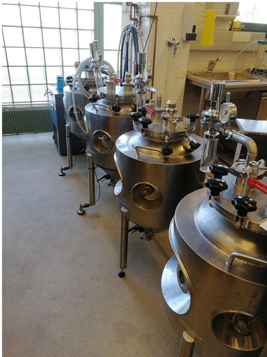
Figure 11. Four fermentation tanks of the microbrewery
