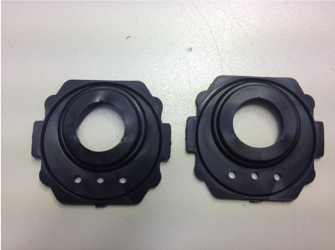
Figure 15 In the picture, you can see some shrinkage in the plastic piece on the left side that needed to be prevented by changing the input values. (Photograph Mikael Hellman, Suunto 2012)
