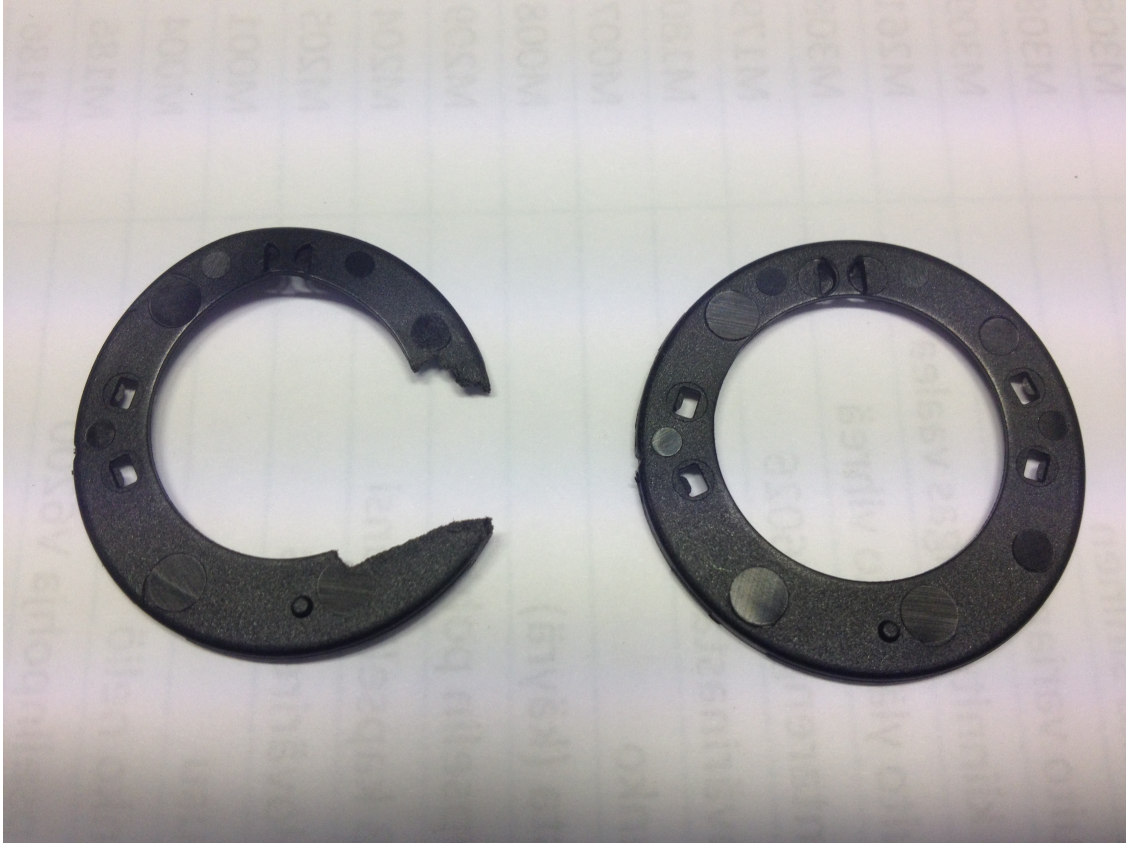
Figure 29 In this picture you can see that the part was not complete. (Photograph Mikael Hellman, Suunto 2012)
