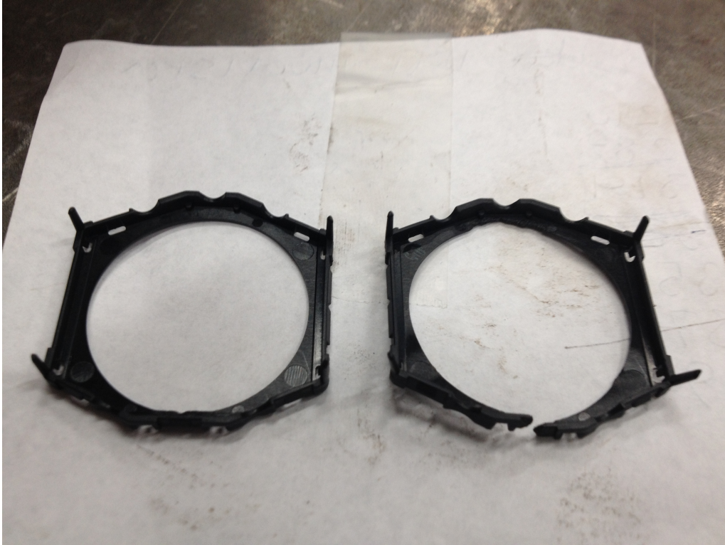
Figure 21 In the picture beneath you can see that the plastic piece was not complete, but needed to be fixed. (Photograph Mikael Hellman, Suunto 2012)
