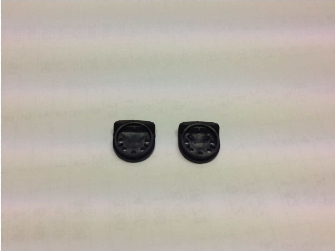
Figure 18 In the picture below you can see some shrinkage in the plastic piece to the right that needed to be prevented. (Photograph Mikael Hellman, Suunto 2012)
