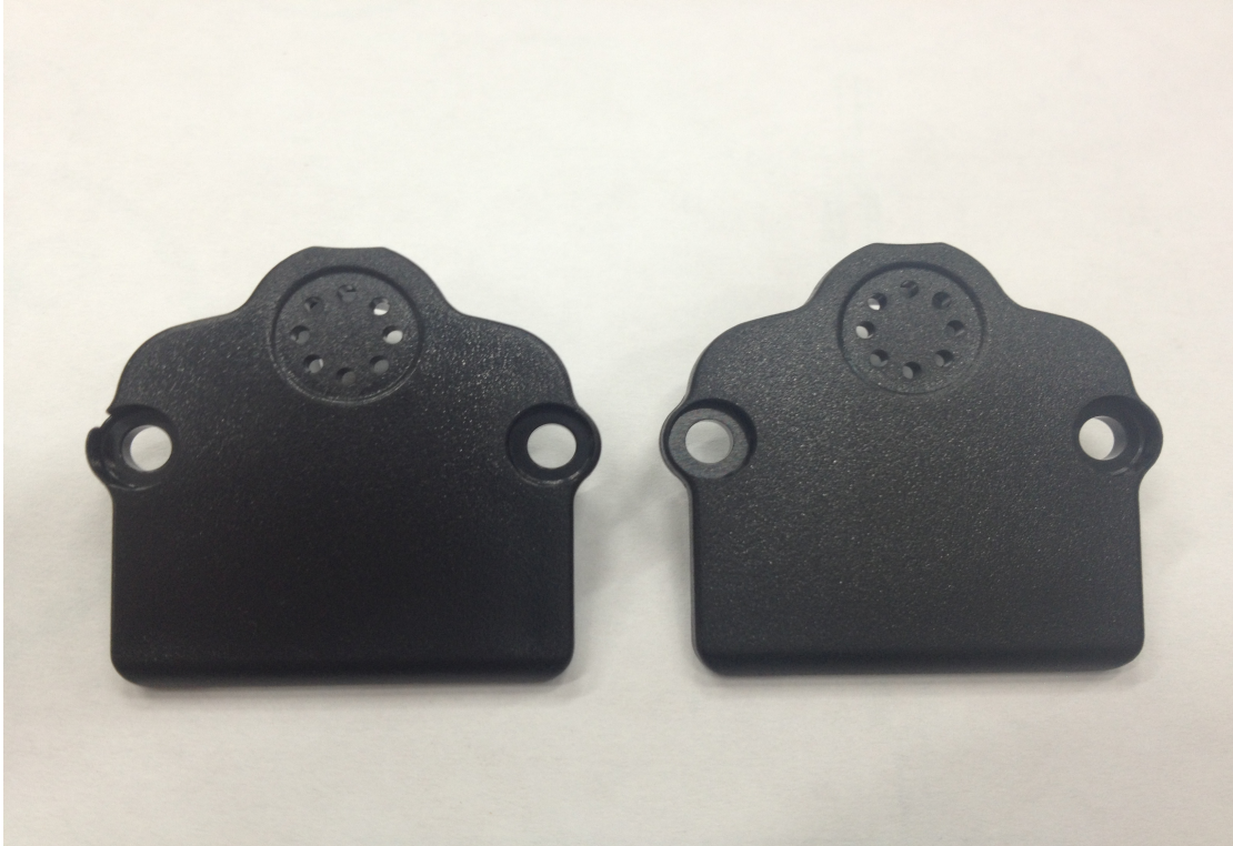
Figure 26 In the picture you can see that the plastic piece to the left is not complete but needed to be fixed. (Photograph Mikael Hellman, Suunto 2012)
