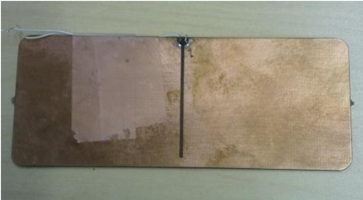
Figure 22 A picture of slot antenna with the G2iL+ chip
