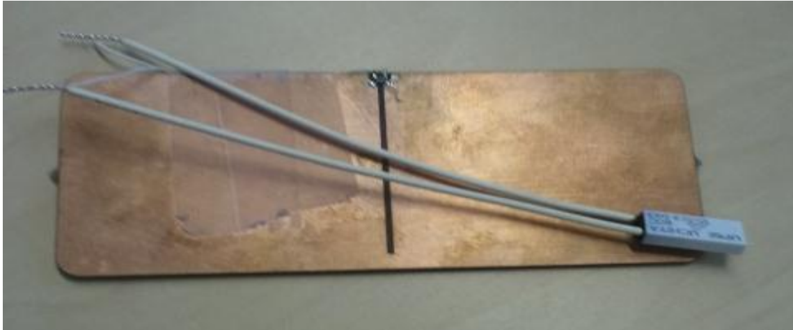
Figure 28 A constructed RFID Temperature smart sensor
