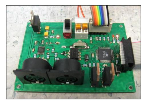
Figure 15 – The MIDI interpreter board. Two MIDI connectors on the lower left side of the board, I2C bus cabling on the right, ATmega16 programming cable on top right. (Photo: Artemis Project 2008)
