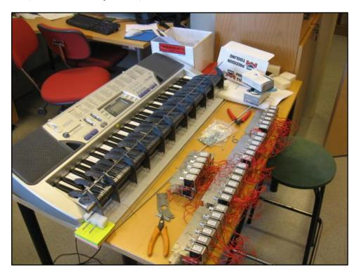
Figure 7 – Incomplete finger mechanics. There are 61 solenoids on the right side of the table. The solenoids were later put into acrylic frames with their respective mechanics controller boards. (Photo: Artemis Project 2008)
