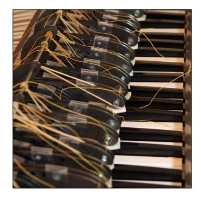
Figure 6 – Finger mechanics placed on top of piano keys. This design was deemed nonfunctional because the fingers did not go down and back up correctly most of the time. This realization came unfortunately too late, this was the reason we came last in the contest. (Photo: Artemis Project 2008)
