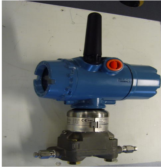
Figure 10 Differential level pressure Transmitter.
