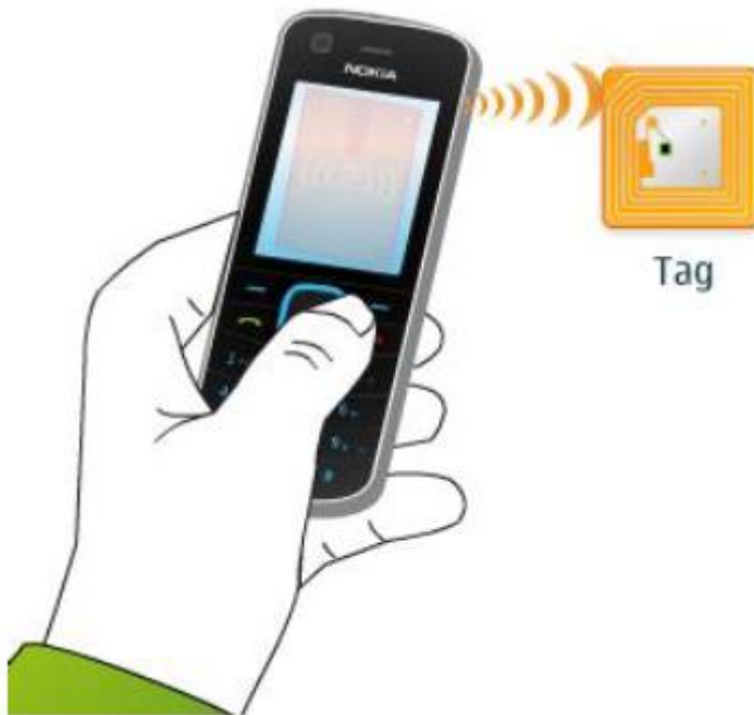
Figure 3: Reader communicating with the tag. Reprinted from Introduction to NFC [8, 2]
