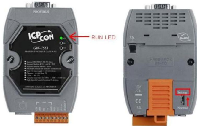
PICTURE 18. Run LED and Normal/Setting switch
