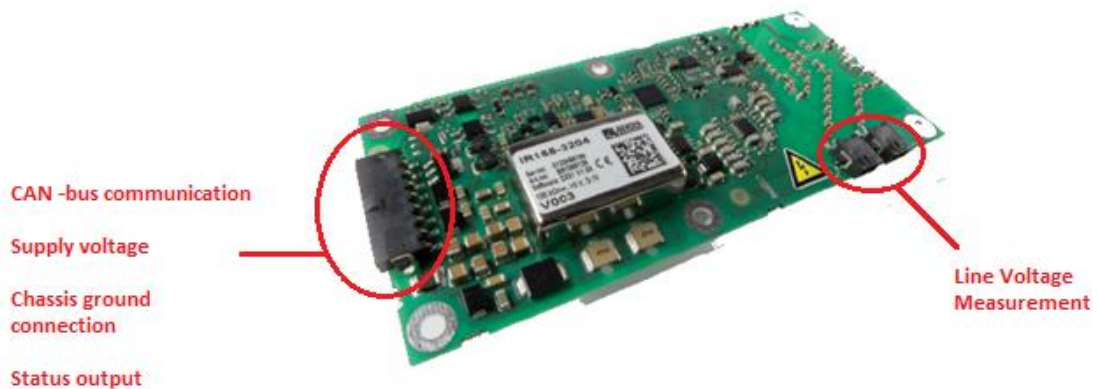
Figure 17. Ground fault detector by Bender
