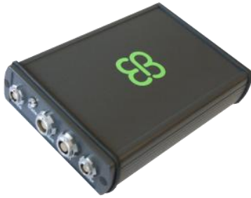
Figure 7. Elektrobit6120 as real-time BMS-master.
