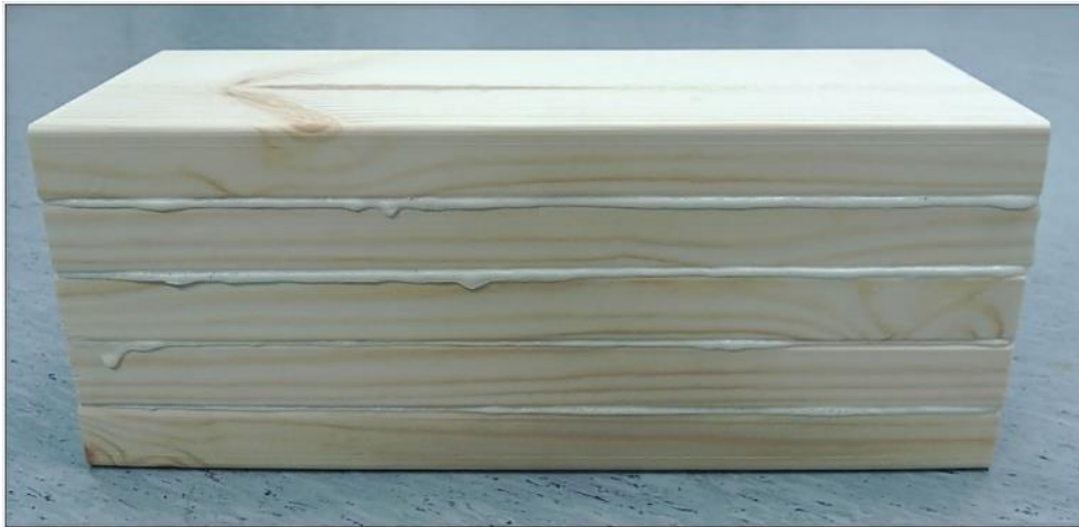
PICTURE 6. Bonded Scots pine assembly for Kiilto EN 302-2 method testing
