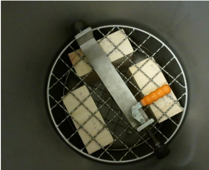
PICTURE 3. SFS EN 391 method B samples inside the pressure vessel
