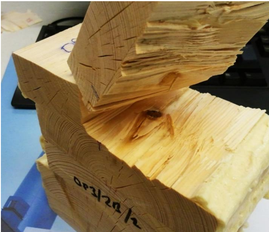
PICTURE 9. A hidden knot in an opened bond line
