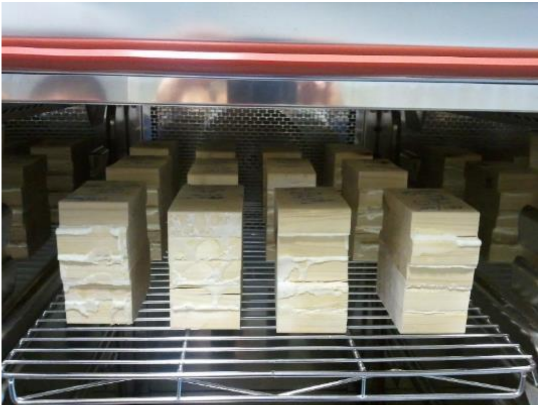
PICTURE 7. Kiilto test method samples drying in the weather chamber
