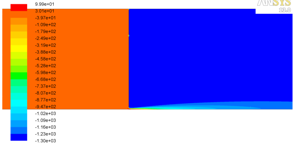
Contours of Total Pressure (pascal) Sep 11, 2012 ANSYS FLUENT 13.0 (2d, dp, pbns, ske)
