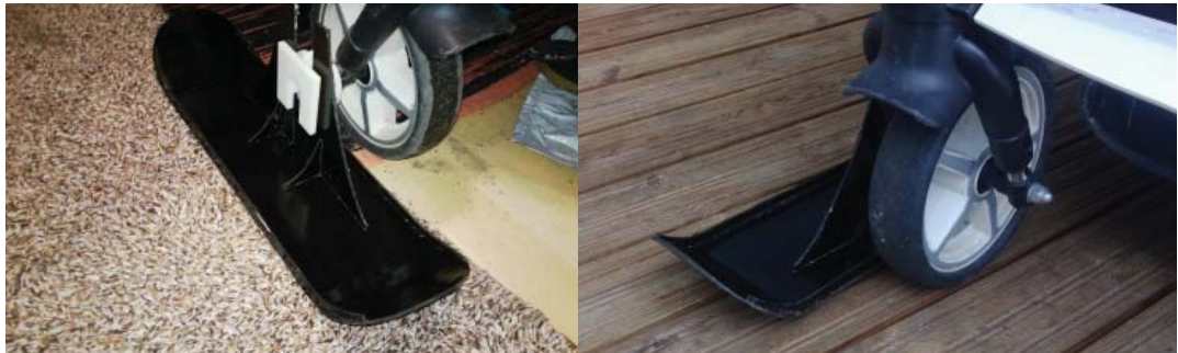
Figure 44: Two photographs from different directions showing the mock-up prototype ski and the 3d printed connection connected to a bolt type connection on a turning pram wheel (Heikkilä 2013)
