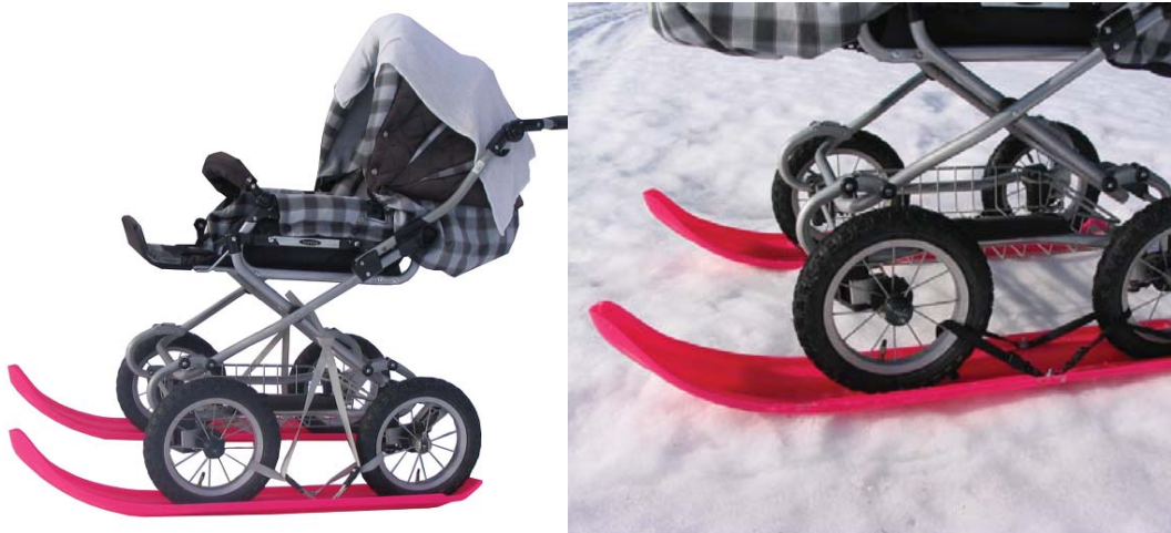
Figure 6: The huge HTSuksee pram skis showing the adorable pink colour and the connection requiring several straps per ski (HTSuksee 2013)
