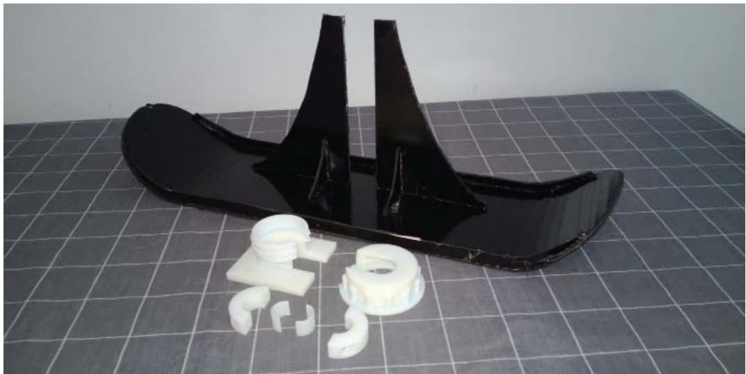
Figure 45: A photograph showing the final connection concept 3d prints and the mock-up prototype of the ski (Heikkilä 2013)
