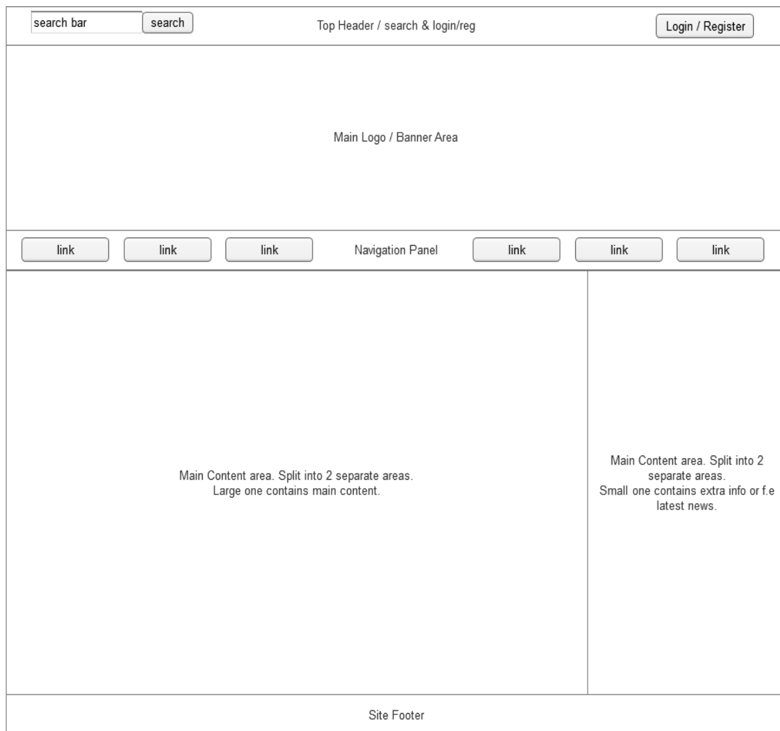
Image: Example of a wireframe sketch which provides the designer the main idea and the main sectioning of the site.
