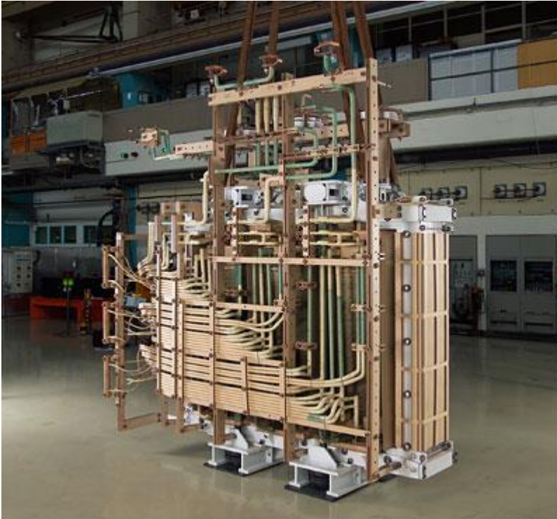
Figure 12. Core-and-coil assembly of a series reactor (made by Siemens)
