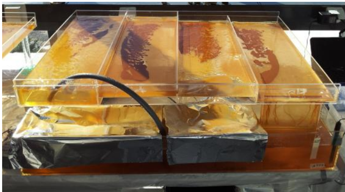
FIGURE 7. Algae Turf Scrubber (Photo, Lorena Lorilla 2013)
