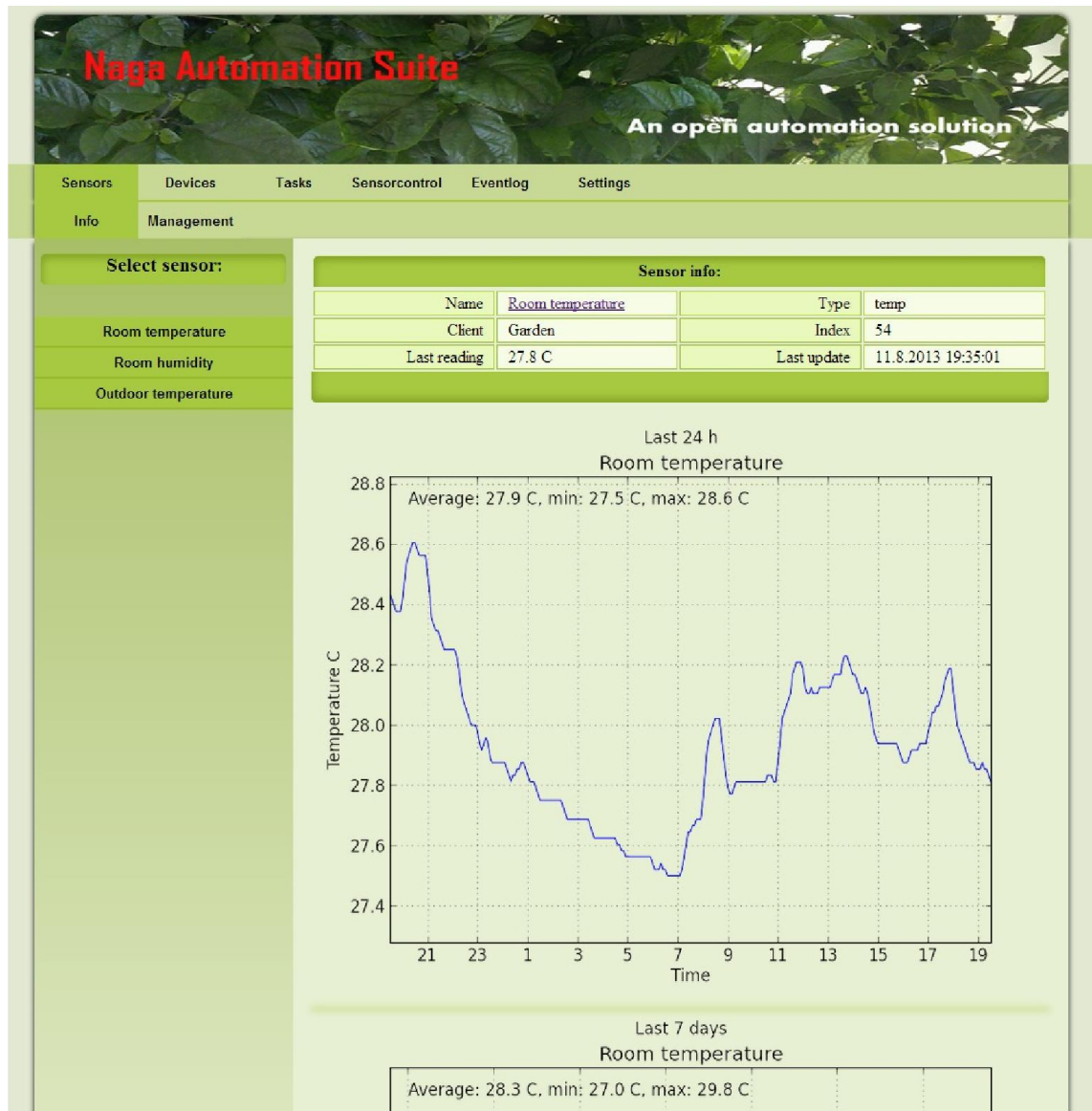
Figure 9 Sensor view of Naga Automation Suite
