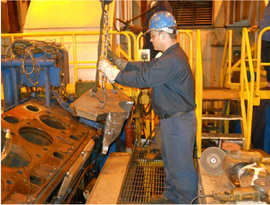
Figure 30. A new cast piece is fitted into place and stitched together with the engine block.
