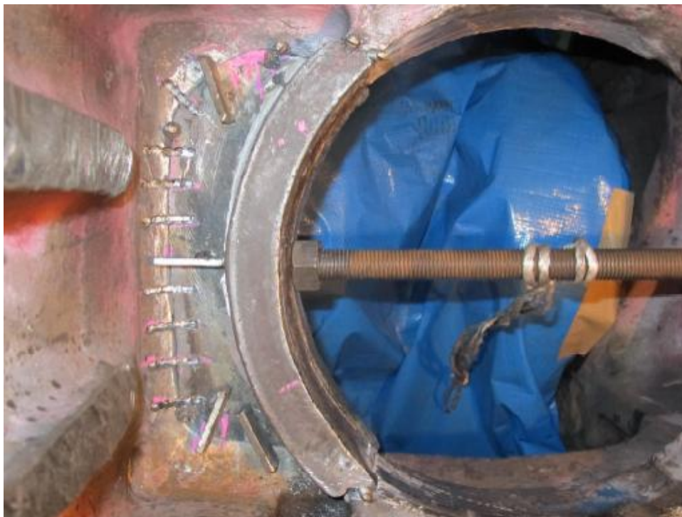
Figure 21. New piece metalocked into place.
