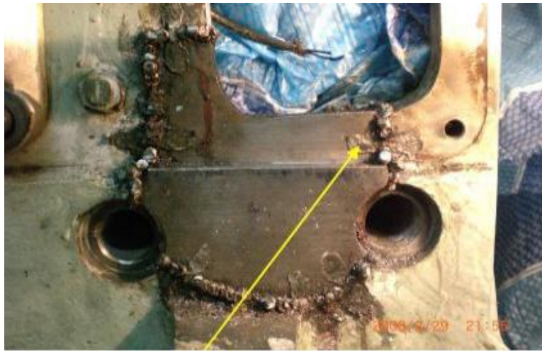
Figure 27. New part locked with keys and metal lace.
