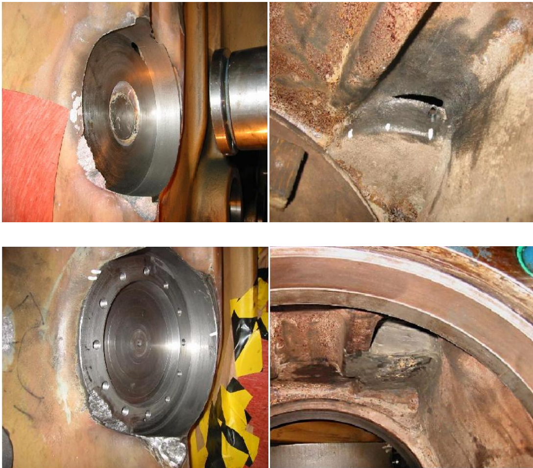
Figure 38. Metallocking of waterspace.
