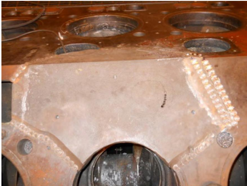
Figure 31. Stitching with pins done.
