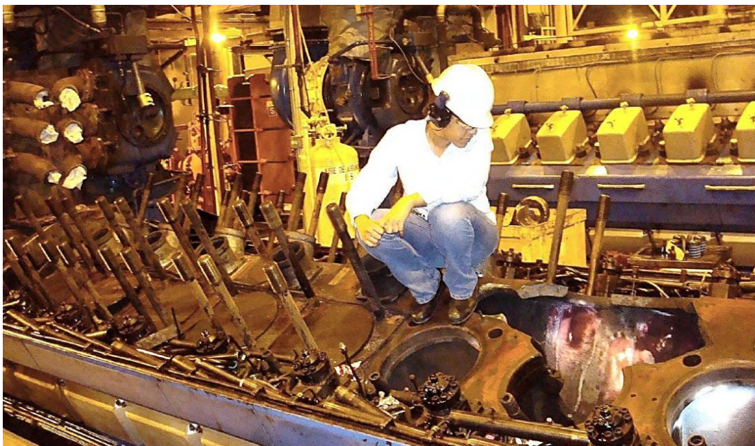
Figure 29. Large piece of the engine block missing.
