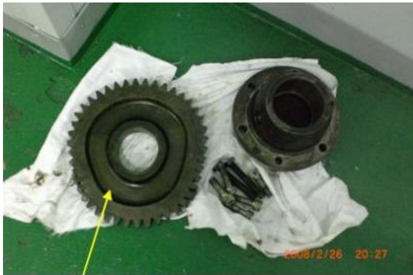
Figure 24. Loosened gear wheel.
