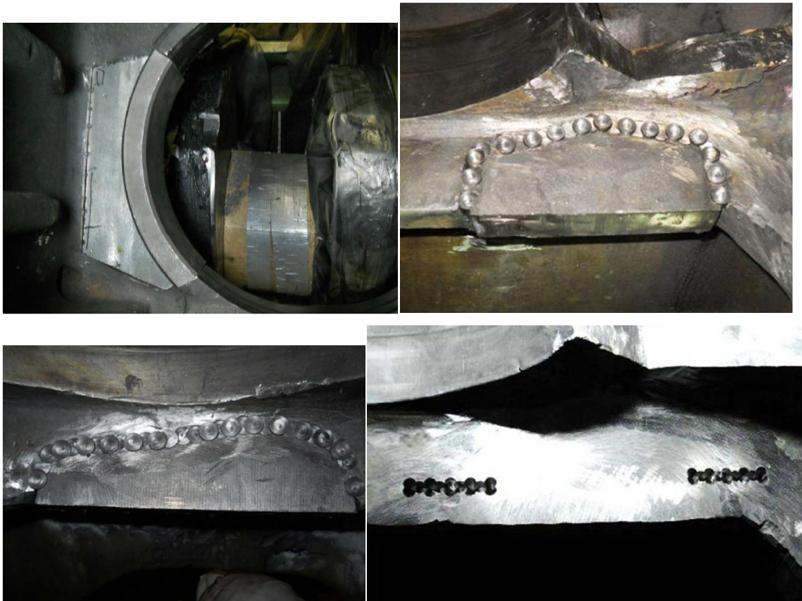
Figure 39. Stitching on 12V32 on Regatta.
