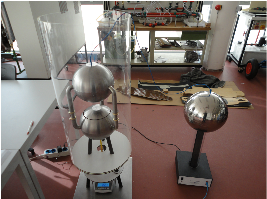
Figure 3: Electrostatic voltmeter connected to Van de Graaff generator in HAN University of Applied Sciences energy laboratory. [Image photographed by Mathias Nummelin (2013) JPEG file.]
