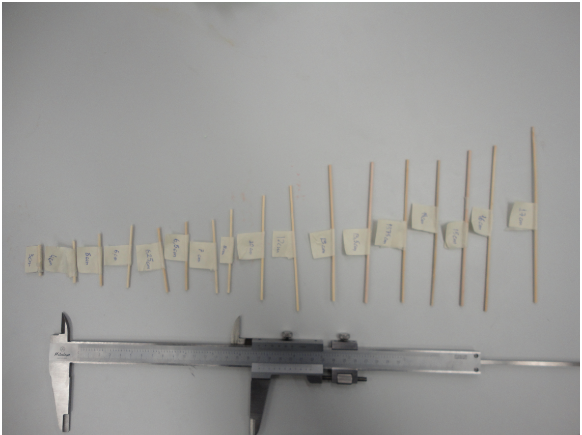
Figure 5: Different size of three pieces for measuring distance between two spheres. [Image photographed by Mathias Nummelin (2013) JPEG file.]
