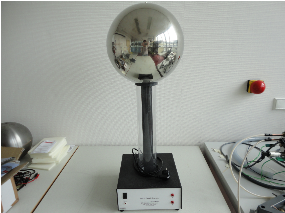
Figure 1: Van de Graaff generator from HAN University of Applied Sciences energy laboratory. [Image photographed by Mathias Nummelin (2013) JPEG file.]
