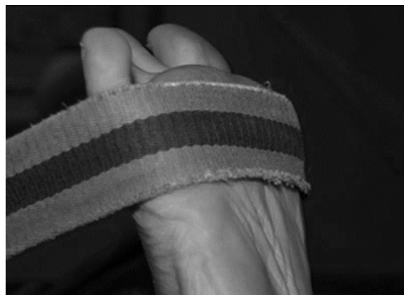
Picture 12. A strap which has begun to fray. Straps need to be designed to take a lot of wear and tear.
