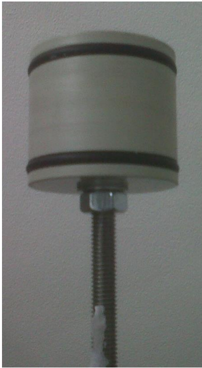
PICTURE 4.3.1: Alternating side branch piston machined from plastic with a separate metal rod (Gyamfi, Katajisto 2014)
