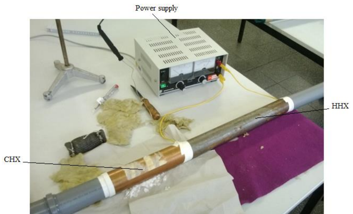
PICTURE 4.4.4: Engine regenerator in the testing facilities Hot and cold reservoir sealed with teflon tape (Tuominen, Mäkinen 2014)
