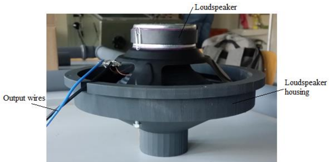
PICTURE 4.3.4: The loudspeaker mounted in the rapid prototyped housing (Tuominen, Mäkinen 2014)
