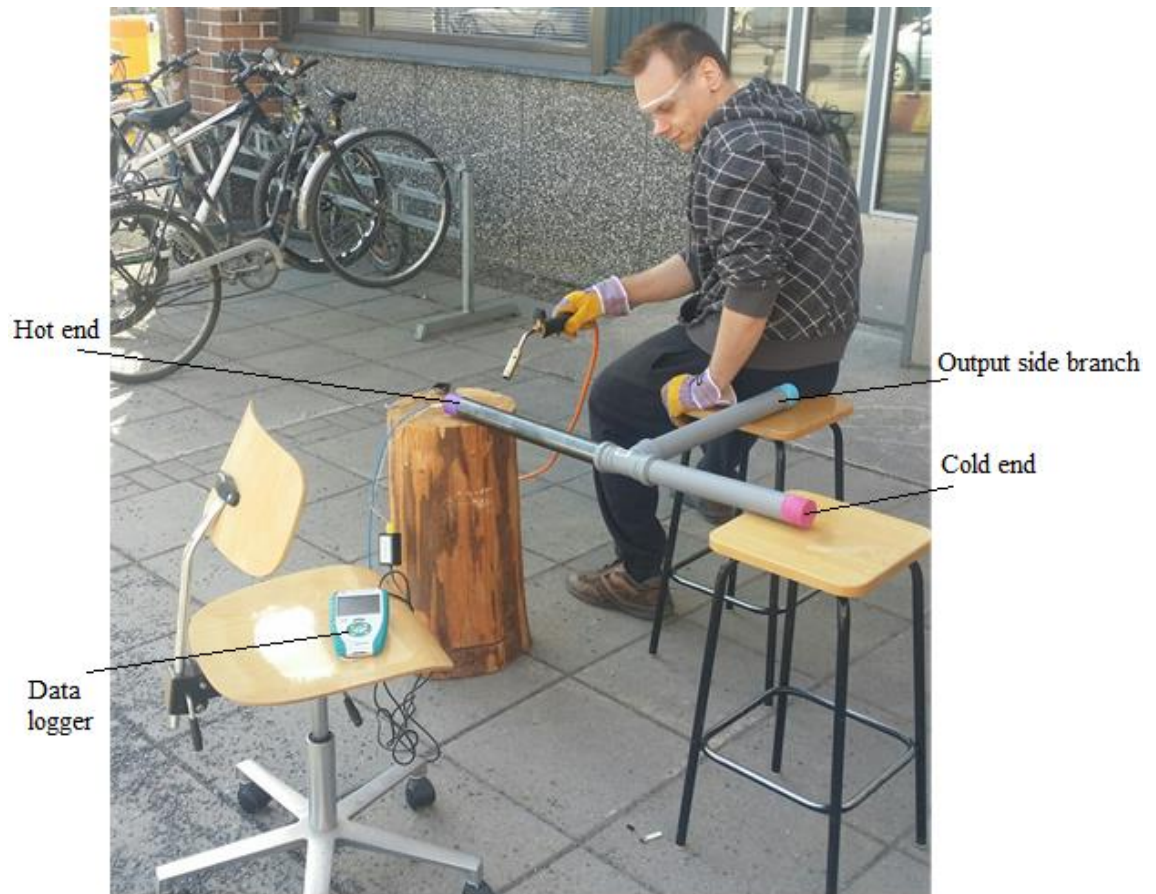
PICTURE 4.4.8: Heating and measuring the T-junction structure (Tuominen, Mäkinen 2014)
