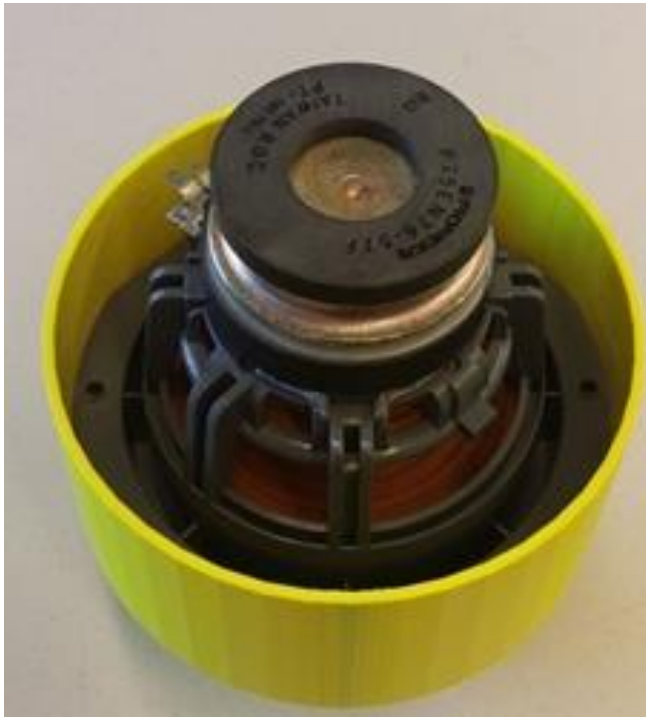
PICTURE 4.4.6: Tampere engines loudspeaker mounted to its housing (Tuominen, Mäkinen 2014)
