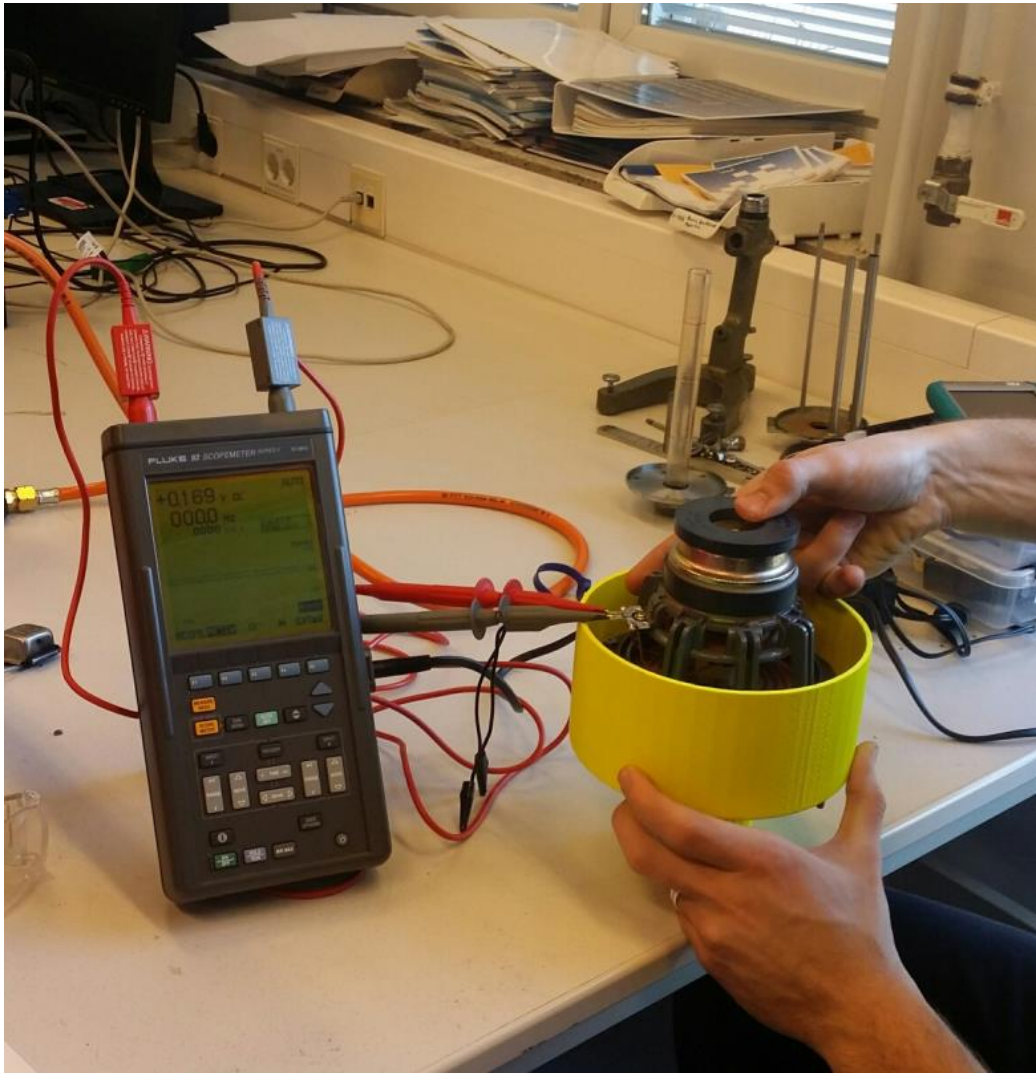
PICTURE 4.4.7: Testing the loudspeaker induction with a Fluke-oscilloscope (Tuomi- nen, Mäkinen 2014)
