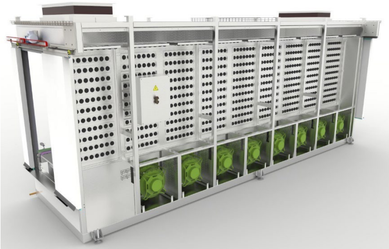
Figure 1. Recirculation of the air in the interior of the tunnel is made by 8 fans situated on the lateral plenum.
