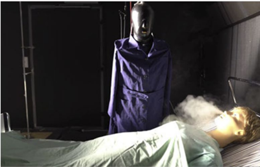
Figure 4. Reduction of HCW exposed to patient exhalation in proximity treatment using protective airflow.
