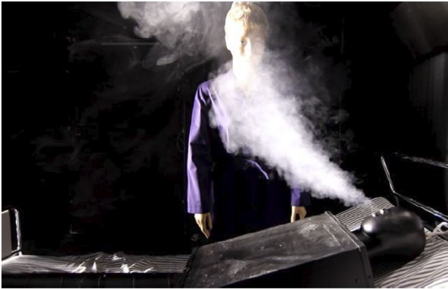
Figure 1. Health care worker's (HCW) exposes to patient exhalation in close proximity treatment situation, mixing ceiling air diffusion (Kalliomäki & Koskela, 2018).
