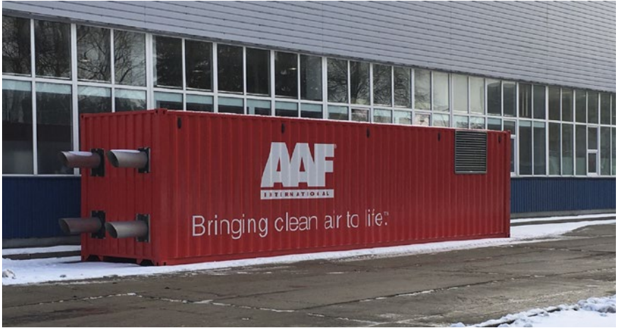
Figure 3. The test container with installed filters located in Latvia. Inside the container are installed two sets of HEPA H14 filters, one with membrane eFRM media and one with traditional glass fiber media. Each filter has a prefilter of class ePM1 55% (F7).
