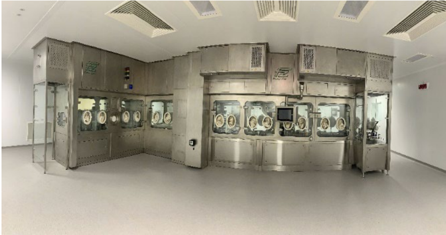
Figure 2. Isolator barrier technology aseptic processing filling line with Grade C surrounding cleanroom.
