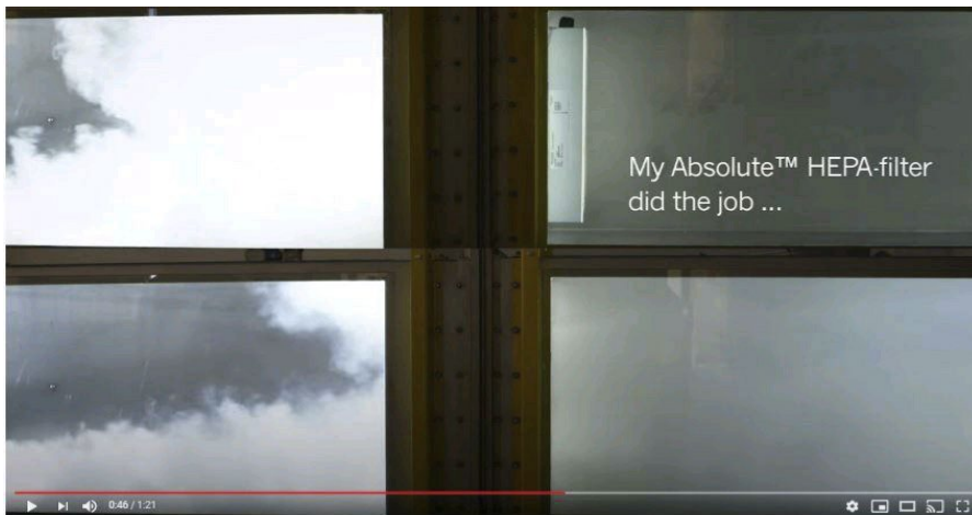
Figure 2. Leak test on a HEPA filter (above) against a so-called True-HEPA filter (below).
