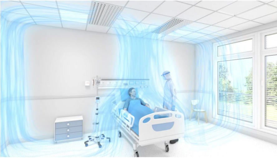
Figure 3. Protective airflow system concept in an isolation room (Halton, 2021).
