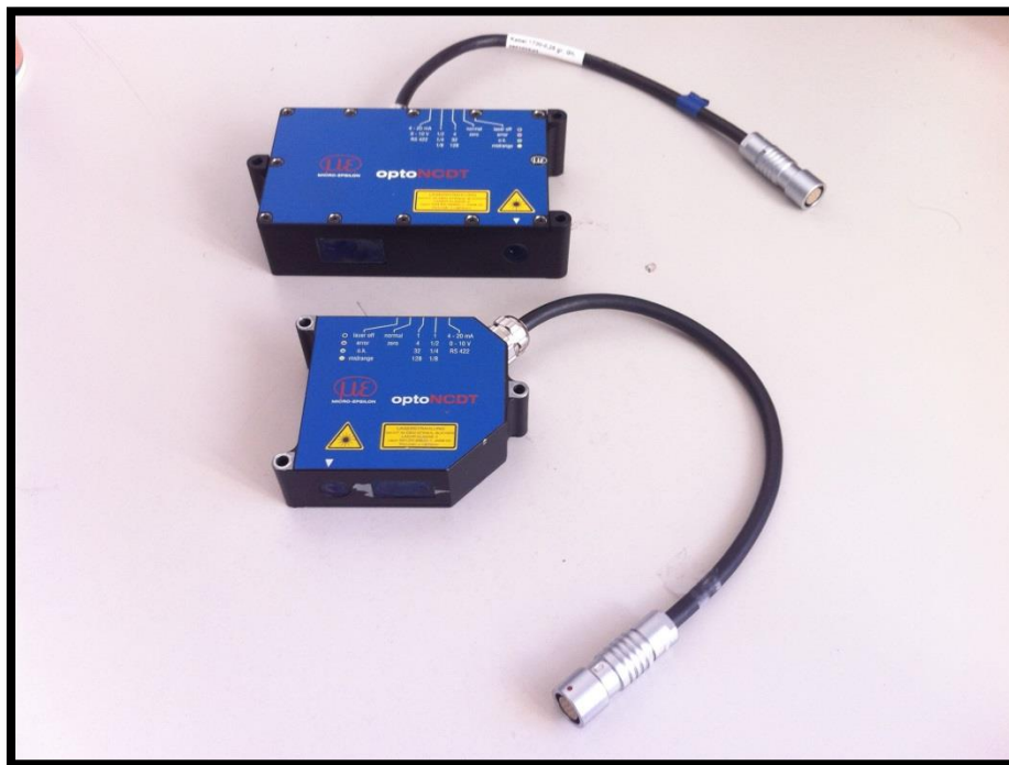
Figure 40 Micro Epsilon laser triangulation sensors, the optoNCDT1700-200 (Below) and the OptoNCDT1700-40 (Top)
