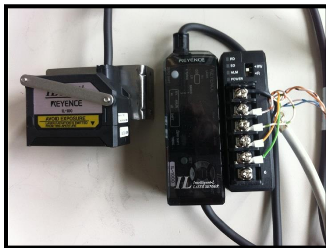
Figure 41 Keyence IL-100 laser triangulation sensor, its amplifier unit and its communicational unit (Left to right)
