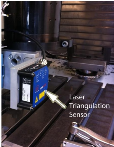
Sketch 4 Laser triangulation sensor attached to the tool of the CNC machine 2
